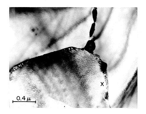
Dark field structure of a specimen aged for 7 hours at  $800^{\rm o}{\rm C}$  showing TiC precipitate at the grain boundary.
