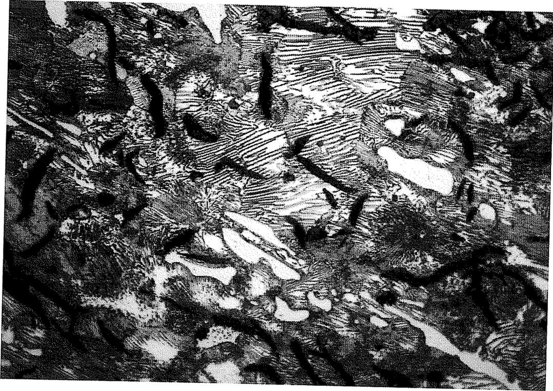
Fig. 3.30 Pore surface structure of cast iron Roller R<sub>1</sub> (X200)
