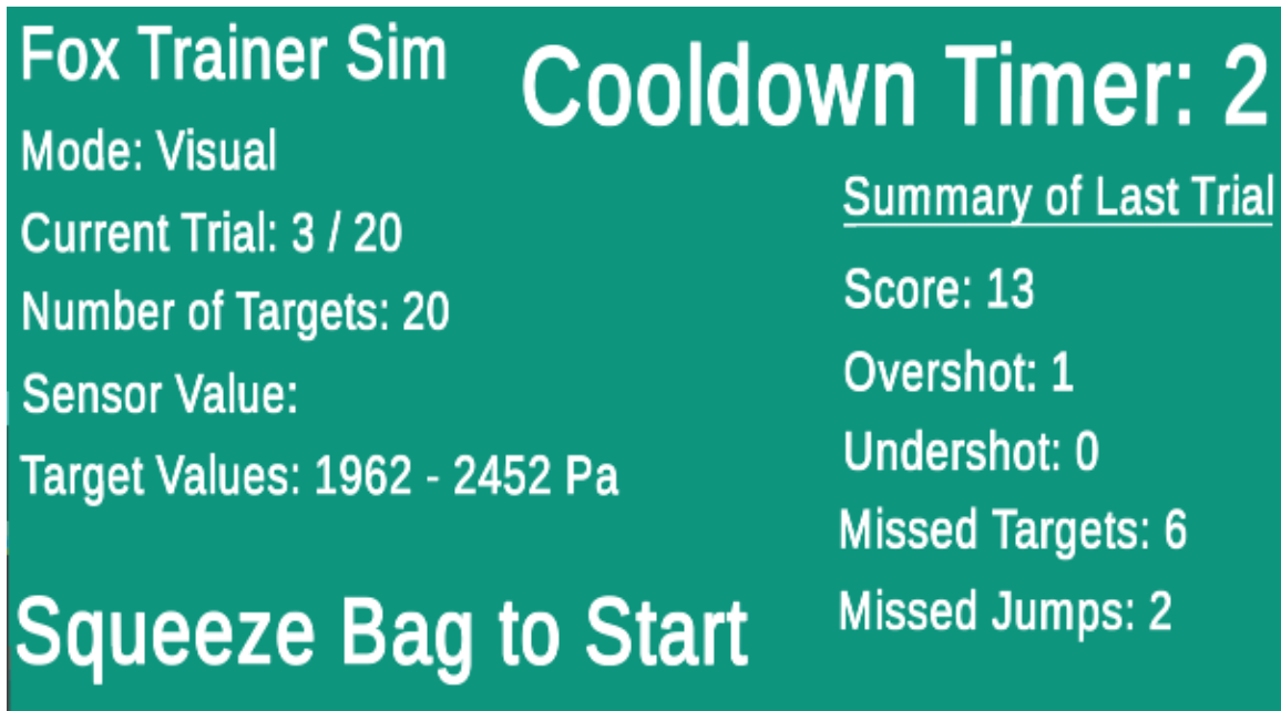
Figure 5.2: The menu screen shown prior to every trial. Compressing the ventilator controls the application.
