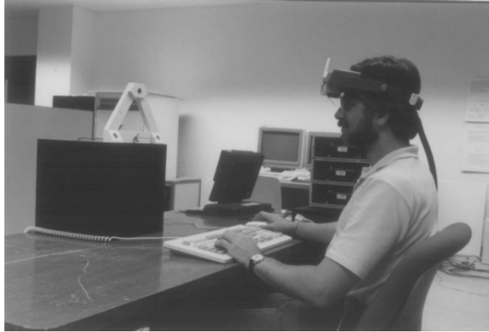
(a) Feiner's window system with an HWDs in 1993 [30]. The large black cube and white triangle are the transmitters for two 3D tracking systems. Tracker receivers are on the head-mounted display, waist, and wrist. (Adopted from [30]. Permission received.)
