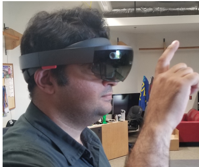
(b) Microsoft HoloLens - One of the latest HWDs released. It requires no external component and all the sensors are implemented with the device.
