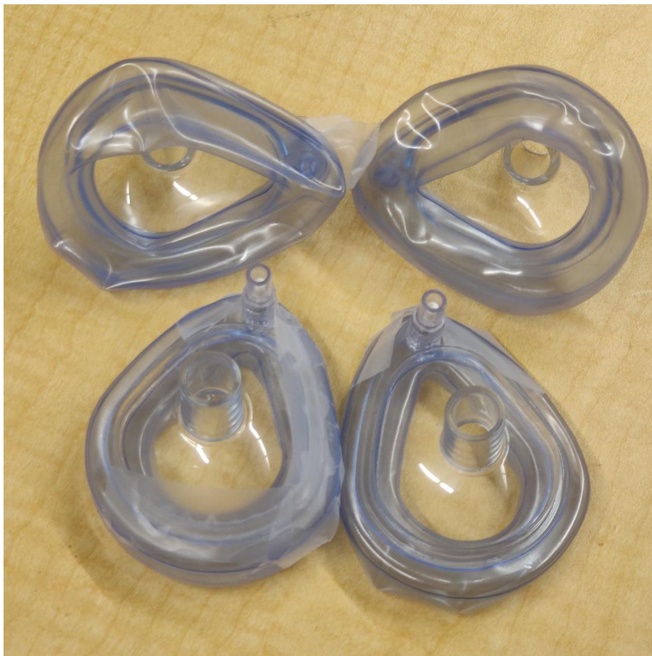
Figure 7.3: Masks damaged due to excessive force
