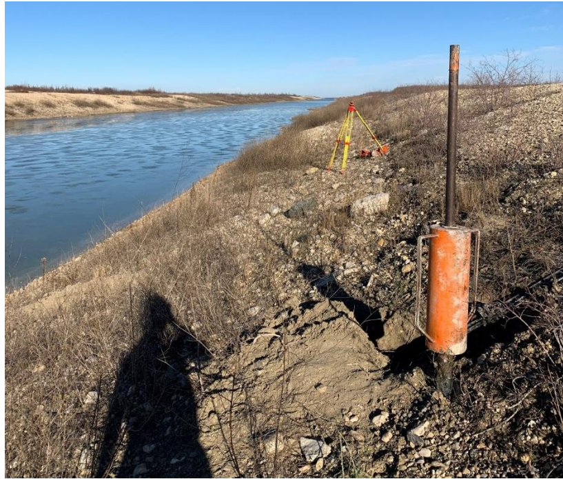
Figure 11: Shelby tube sample extraction near inlet of LSMEOC
