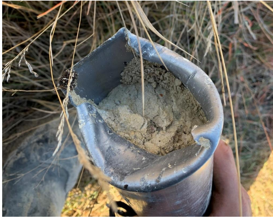
Figure 8: Deformed bevelled (bottom) edge of Shelby tube after sample extraction
