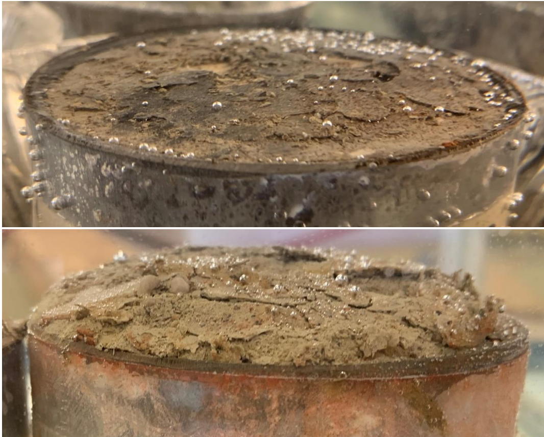
Figure 35: Minor (top) and major (bottom) slaking – Sample Location R1-L7
