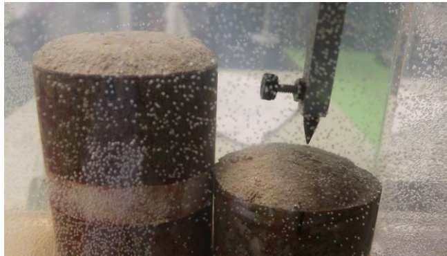
Figure 32: Point gauge used to measure vertical displacement (swelling) of air-dried reconstituted (left) and intact (right) St. Laurent till samples.
