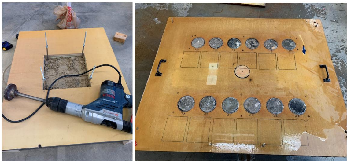
Figure 19: Reconstituted block sample panel (left) and Shelby tube “puck” sample panel (right)
