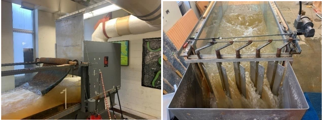
Figure 17: Variable slope flume headwater box (left) and tailwater gate (right)
