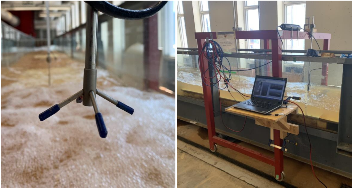
Figure 20: ADV transducer (left) and transducer mounted to point gauge and movable frame with laptop for recording data (right)
