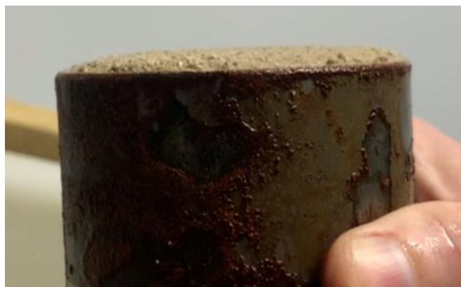
Figure 31: Swelling of reconstituted St. Laurent till sample submerged at in-situ moisture content
