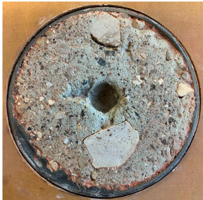
Figure 38: Intact till sample with centre pit drilled prior to testing
