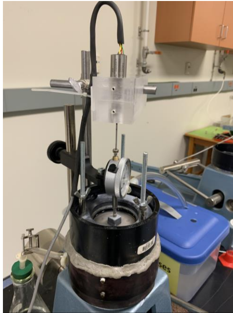
Figure 30: Submerged Shelby tube puck sample with LVDT to measure vertical displacement
