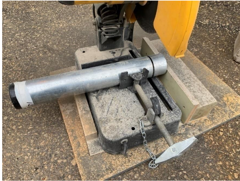
Figure 13: Shelby tube being cut by chop saw with masonry blade and jig for cutting 50 mm lengths
