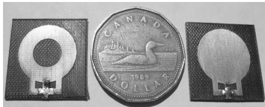
Fig. 3.37 Circular monopole antennas of Fig. 3.8a and Fig. 3.8c etched each on a 22 \times 22 \text{mm}^2 substrate with \epsilon_r=2.5 , height=0.8mm. Antennas are compared to the Canadian Dollar Coin before being mounted on the Aluminium ground plane
