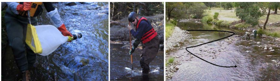
Various invertebrate sampling pictures: kicknet showing detachable cup; person collecting benthic sample using kicknet; kicknet pattern in river
