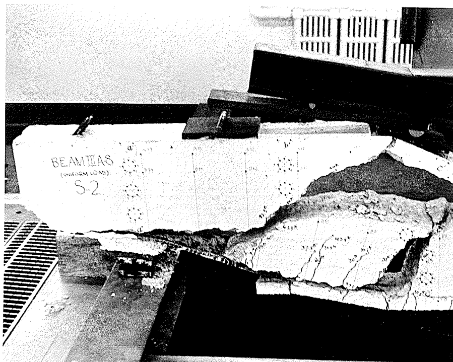
FIG. 61 FAILURE OF BEAM IIIA-8
