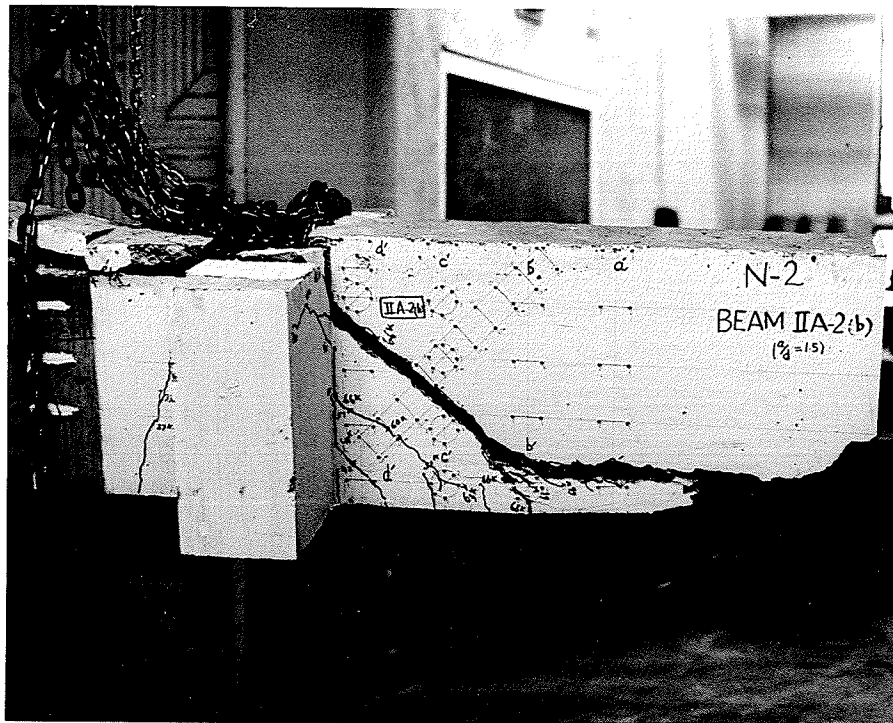
FIG. 50 - BEAM IIA-2 (b) AT FAILURE - END N2
