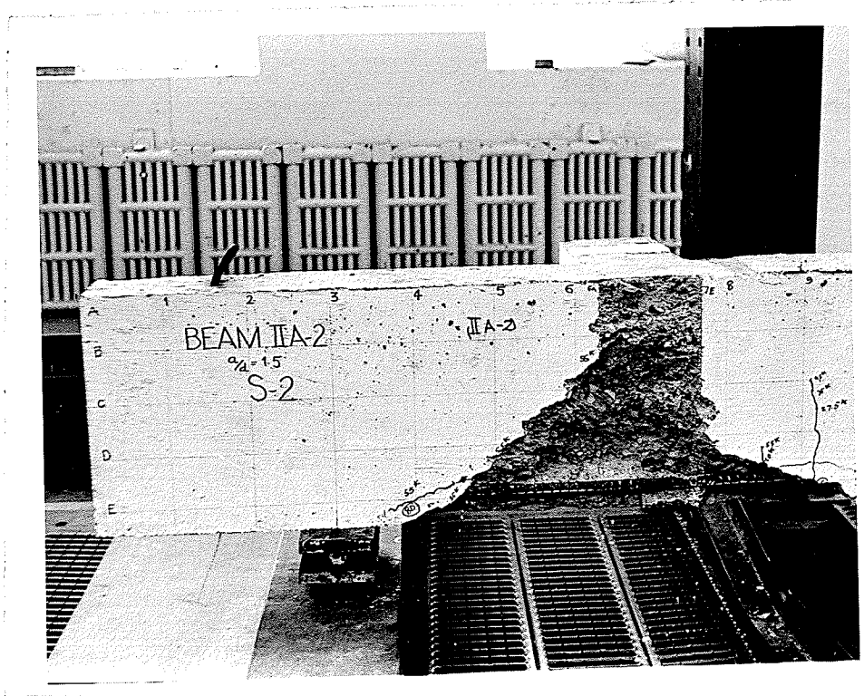
FIG. 48 FAILURE OF BEAM IIA-2 AT THE JUNCTION OF SECONDARY BEAM TO THE MAIN BEAM
