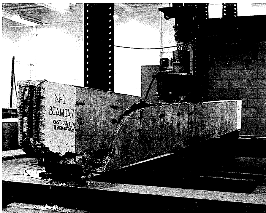
FIG. 35 DIAGONAL FAILURE OF BEAM IA-7
