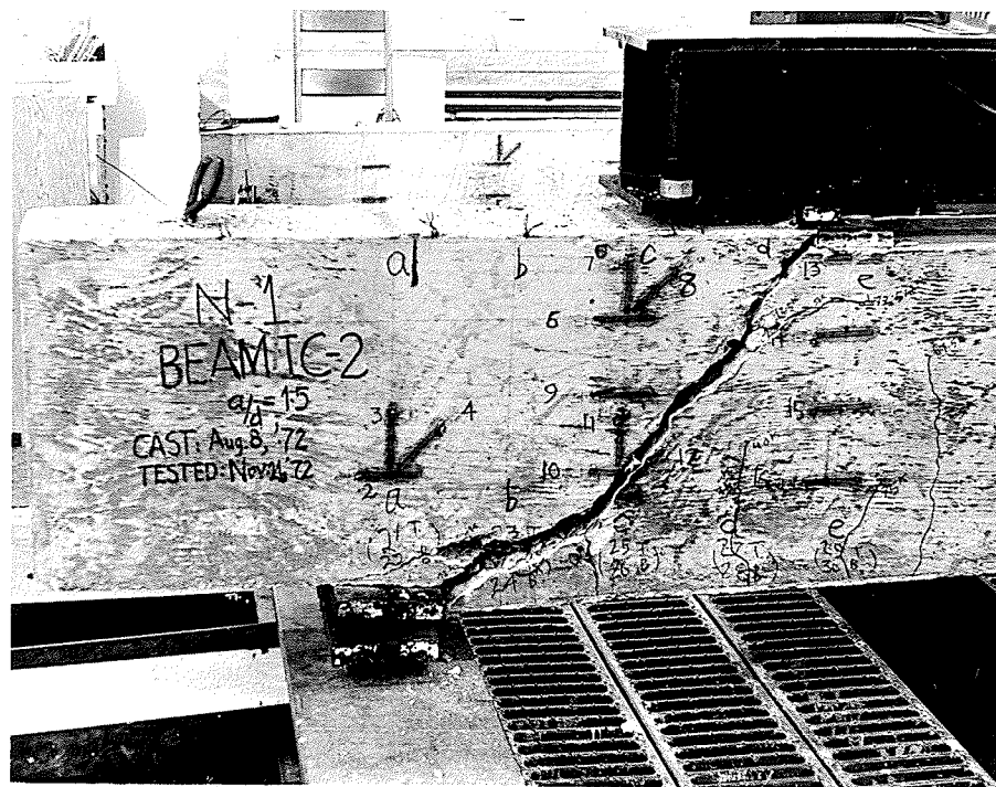
FIG. 43 FAILURE OF BEAM IC-2
