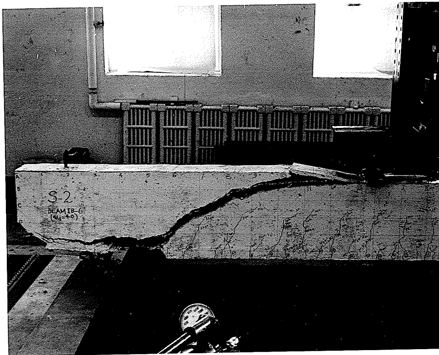
FIG. 42 DIAGONAL TENSION FAILURE OF BEAM IB-6 (END S2)
