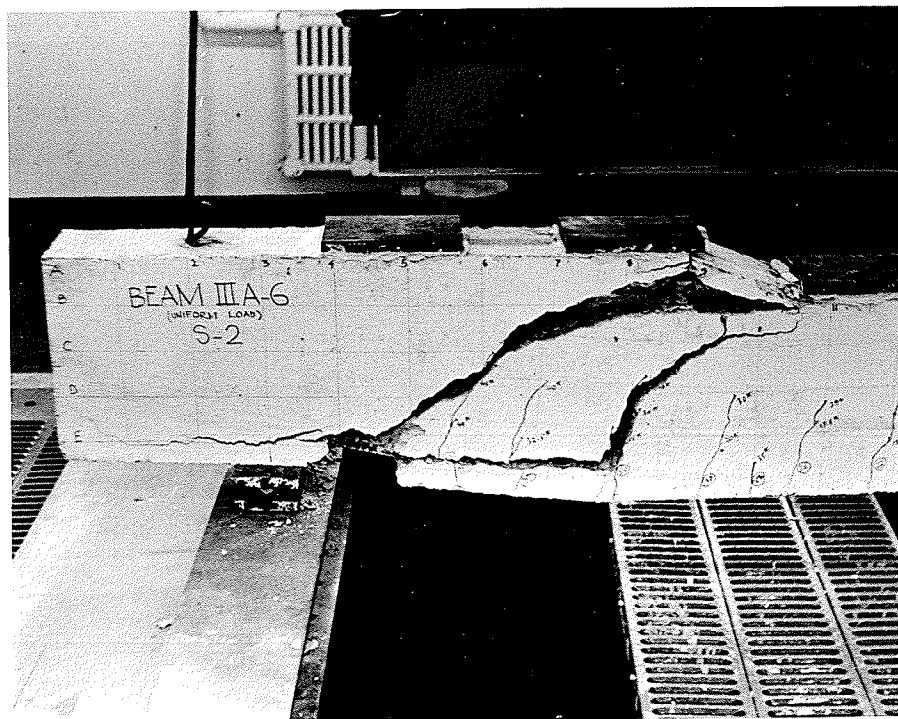
FIG. 60 FAILURE OF BEAM IIIA-6
