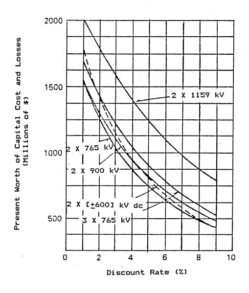
FIGURE 7. Cost Comparison with Varying Losses [19].
