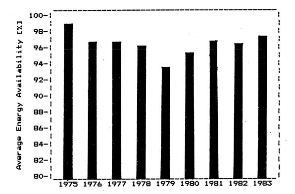
FIGURE A1-3. Average Energy Unavailability of Mercury-Arc Valve Stations [31].
