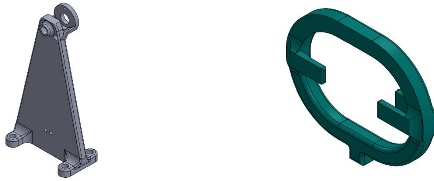
(a) (b) Figure 12: (a) Link 0 supporting serial links, (b) yoke.
