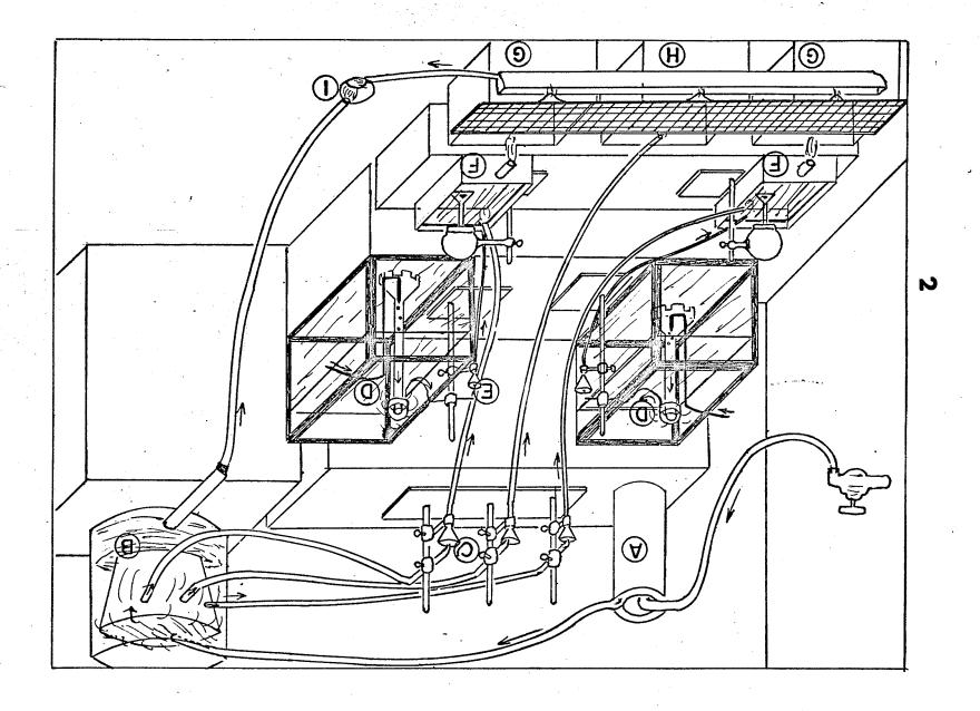
diluent flow-regulating mechanisms (Fig. 2C) of the individual aquaria. Each flow-regulator consists of:
