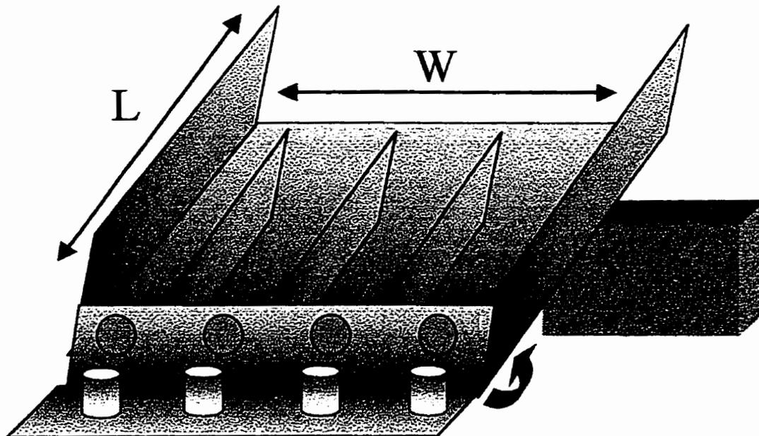
**Figure 5.** A schematic representation of the homemade multi-unit animal holder used for mouse saliva collection. The unit was constructed out of extra-strength cardboard with a length (L) of 32.5 cm, a width (W) of 42 cm and a diameter of 3.5 cm for each window. The saliva was collected into the glass vials placed directly underneath each window. A small box was used to elevate the apparatus at a 10-20° angle (blue arrow).
