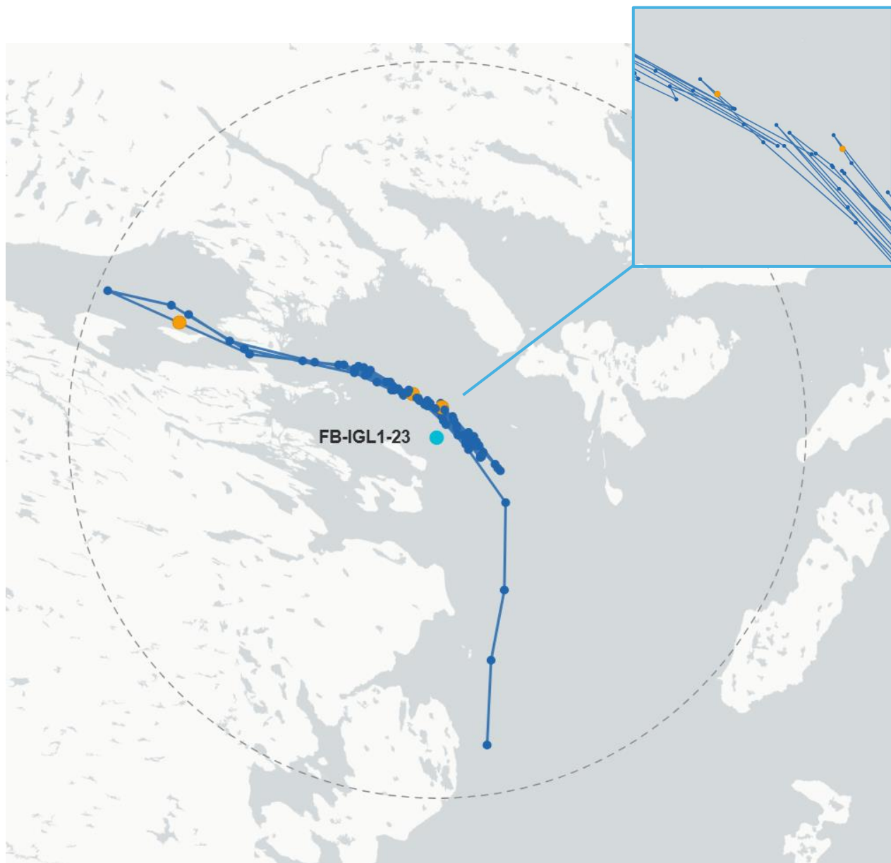
Figure S3.4 Example of interpolated AIS positions (blue points) and three interpolated positions (orange points) for transit 1 of the Icebreaker (ship ID: 439469789) in September 2023. The inset (top right) shows a close-up of the two interpolated positions nearest the hydrophone FB-IGL1-23 (cyan point). The dashed circle represents the 100 km buffer zone used in the study.
