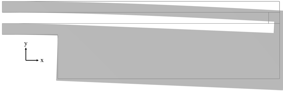
(b) Top view of the actuator in operation. Deformation is exaggerated.
