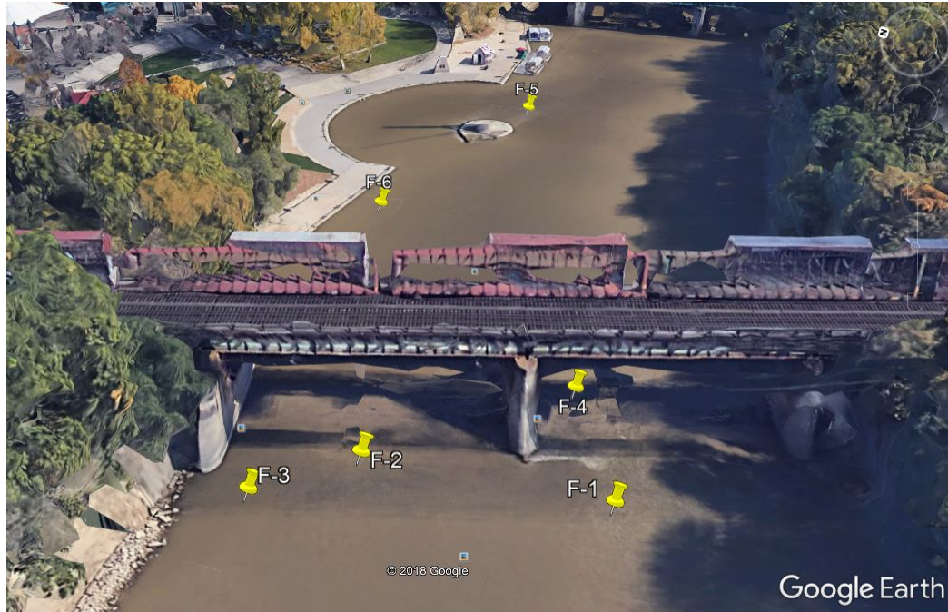
Figure 4.15: Location of the surface measurement points on the Assiniboine River at the Forks in Winnipeg. Multiple points are selected to capture the range of velocities occurring in the river.
