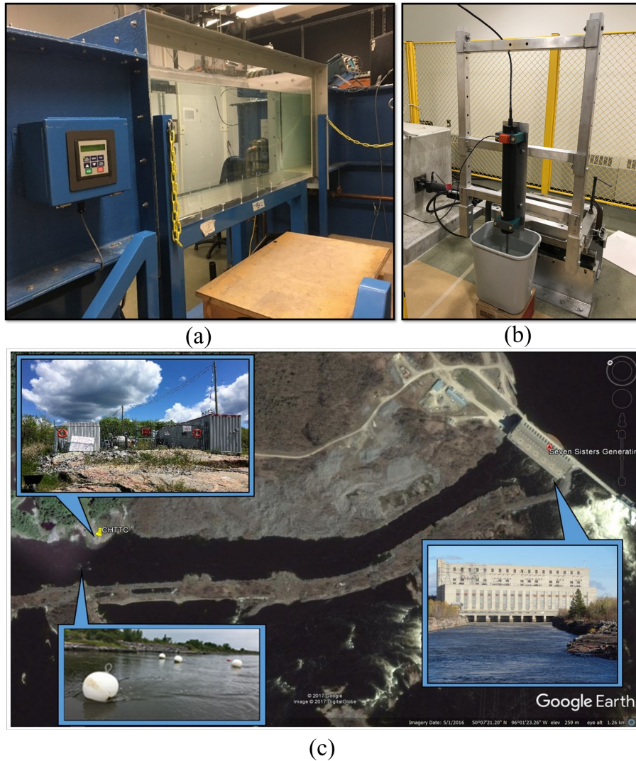
Figure 3.4: Test facilities: (a) Test section of water tunnel, (b) shaker table with ADV mount assembly with IMU located inside the instrument with probe immersed in a water container, and (c) Google Earth view of the CHTTC site showing the location of seven sister dam, CHTTC site office, and the buoys
