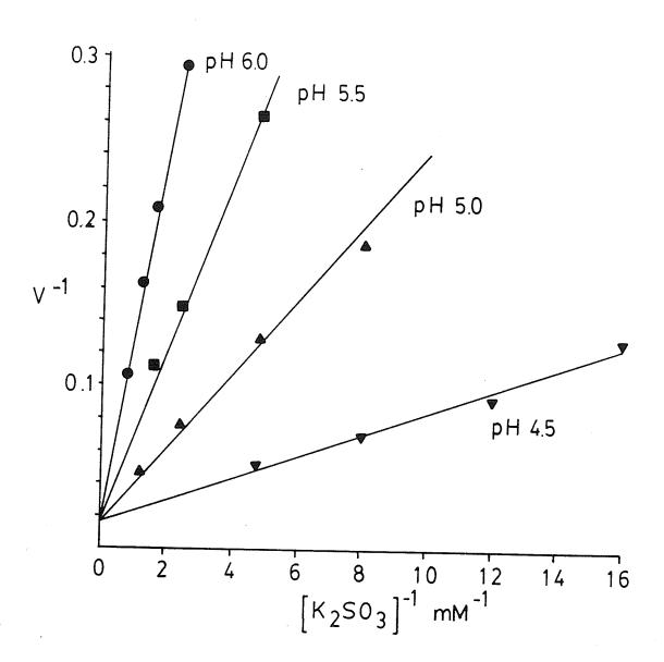
Figure 18. Effect of pH on the double reciprocal plot of sulfite oxidation rates and sulfite concentrations by SM-7. SM-7 mine isolate (Lizama and Suzuki, 1987) cells (1 mg wet cells) were washed and assayed at 50 mM potassium phosphate buffer as described in Materials and Methods. K<sub>m</sub> and V<sub>max</sub> values are listed in Table 5.
