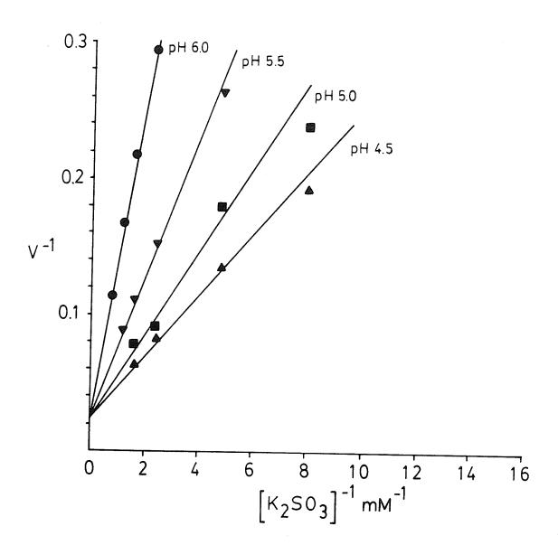
Figure 17. Effect of pH on the double reciprocal plot of sulfite oxidation rates and sulfite concentrations by SM-6. SM-6 mine isolate (Lizama and Suzuki, 1987) cells (1 mg wet cells) were washed and assayed at 50 mM potassium phosphate buffer as described in Materials and Methods. K<sub>m</sub> and V<sub>max</sub> values are listed in Table 5.
