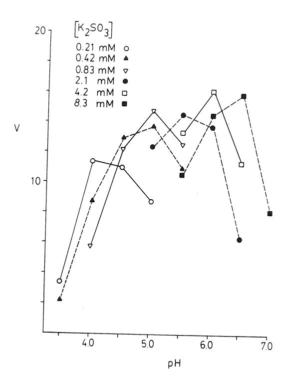
Table 1. Chemical oxidation rates for sulfite in potassium phosphate buffer at varied pH
