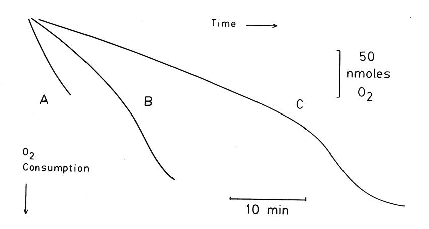
Figure 8. Effect of potassium phosphate concentration on sulfide oxidation by T. thiooxidans in washing and assay. Sulfide oxidation was followed as described in Materials and Methods with 7.5 μl of 20 mM sodium sulfide to start the reaction with 1 mg wet cells. Cells were washed in pH 2.3 50 mM (A and B) or 500 mM (C and D) potassium phosphate and assayed in 50 mM (A and C) or 500 mM (B and D) potassium phosphate at pH 2.3.
