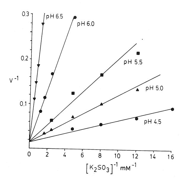
Figure 10. Effect of pH on the double reciprocal plot of sulfite oxidation rates and sulfite concentrations (Starkey's No.1 washed cells). Thiobacillus thiooxidans cells (1 mg wet cells) were washed and resuspended in Starkey's No. 1 medium, pH 2.3 as described in Materials and Methods.  $K_m$  and  $V_{max}$  values are listed in Table 4.
