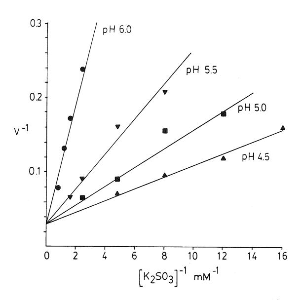
Figure 12. Effect of pH on the double reciprocal plot of sulfite oxidation rates and sulfite concentrations (HP medium grown and washed cells). Thiobacillus thiooxidans cells (1 mg wet cells) were grown in HP medium (Lizama and Suzuki, 1988) for 4 days. Cells were washed and resuspended in same, pH 2.3 as described in Materials and Methods.  $K_m$  and  $V_{max}$  values are listed in Table 4.
