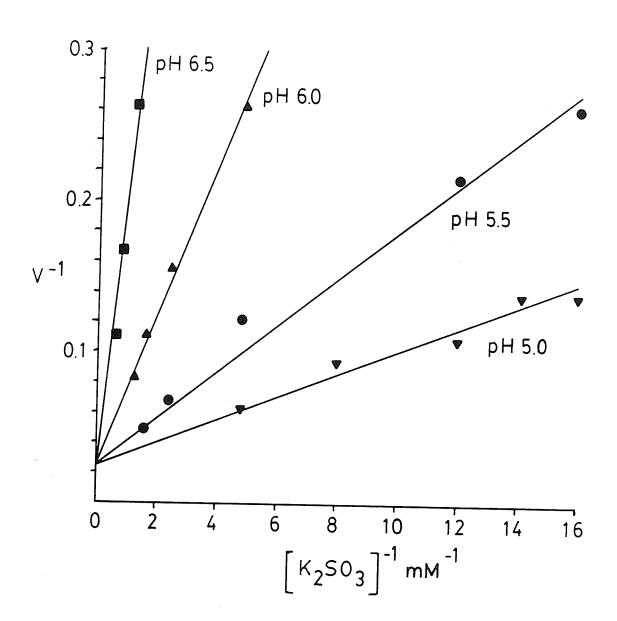
Figure 13. Effect of pH on the double reciprocal plot of sulfite oxidation rates and sulfite concentrations (HP medium grown cells washed in potassium phosphate at pH 2.3). Thiobacillus thiooxidans cells (1 mg wet cells) were grown in HP medium (Lizama and Suzuki, 1988) for 4 days. Cells were washed and resuspended in 50 mM potassium phosphate buffer, pH 2.3 as described in Materials and Methods. K<sub>m</sub> and V<sub>max</sub> values are listed in Table 4.
