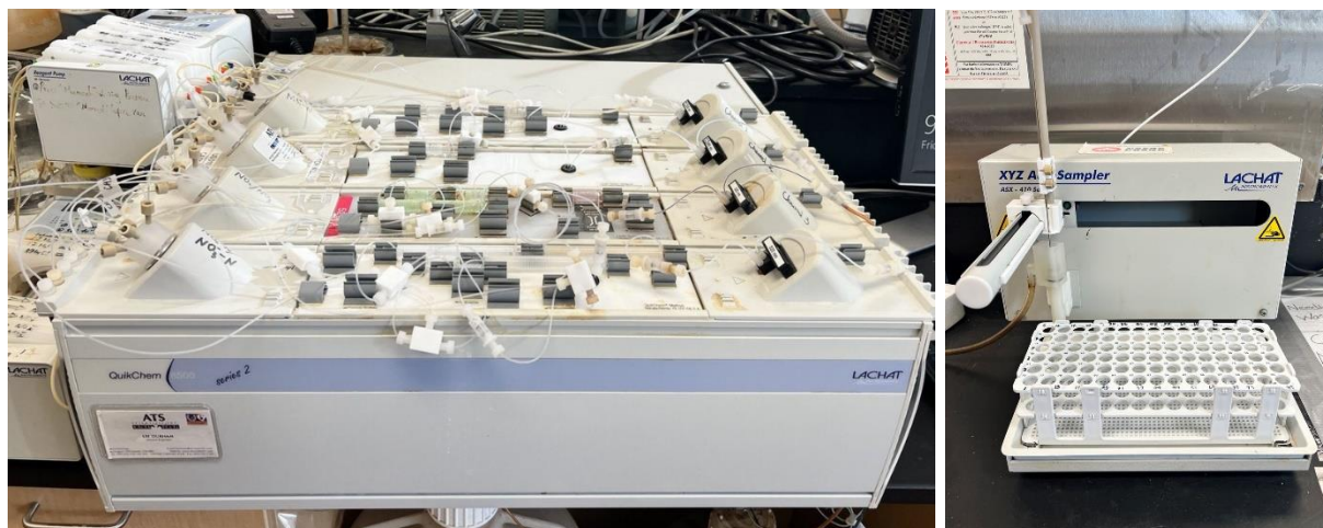
Figure 3.6. a) Flow injection analysis instrument and, b) Auto sampler
