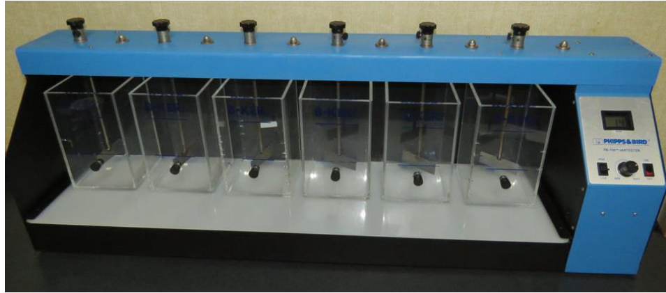
Figure 3.1. Jar test apparatus
