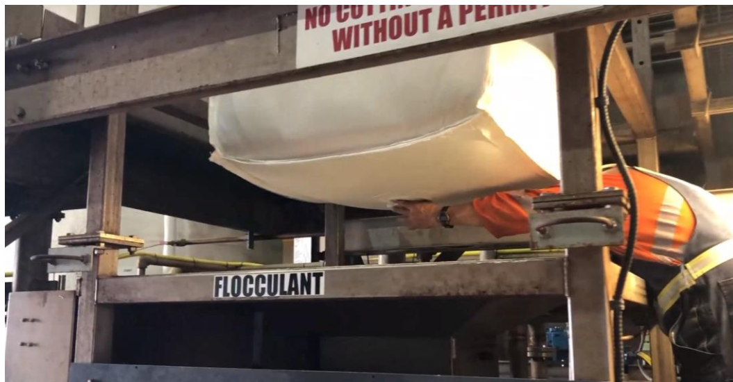
Figure 2: Flocculant bag being opened by operator
