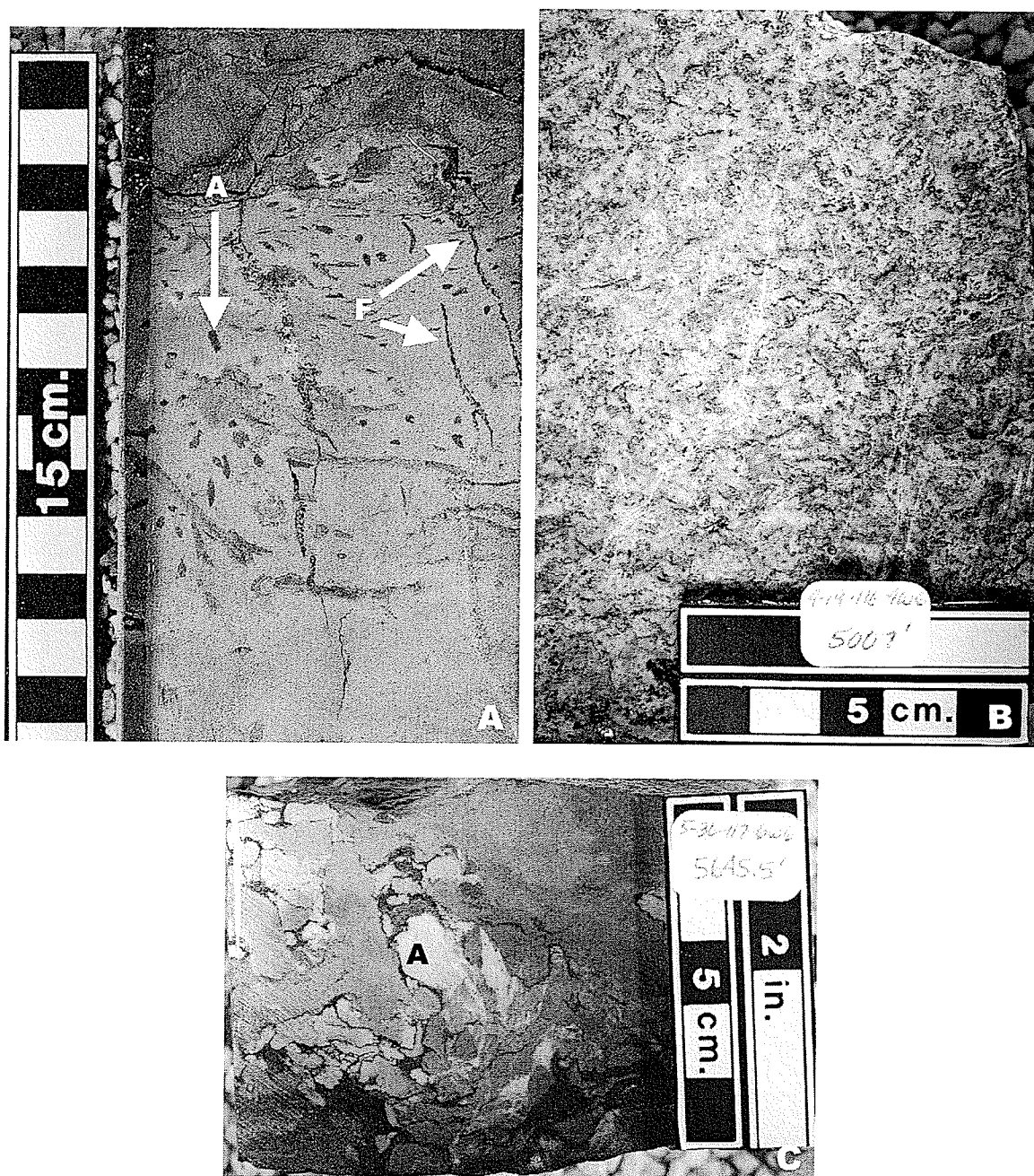
Figure 3.13 Core photos of lithofacies I: non-fossiliferous dolomudstone. A) Massive dolomudstone showing abundant anhydrite laths (A) and dolomite-filled fractures (F). 4-9-109-8 W6M, 2042.2 m (6700.11 ft). B) Haloturbated dolomudstone. Buff-colored areas are pseudospar and nonplanar dolomite. Darker grey areas are coarse to very coarse-crystalline, subhedral anhydrite. 4-19-116-4 W6M, 1526.1 m (5007 ft). C) Brecciated dolomudstone exhibiting patches of extremely coarsely crystalline anhydrite (A). 5-36-117-6 W6M, 1720.8 m (5645.5 ft).
