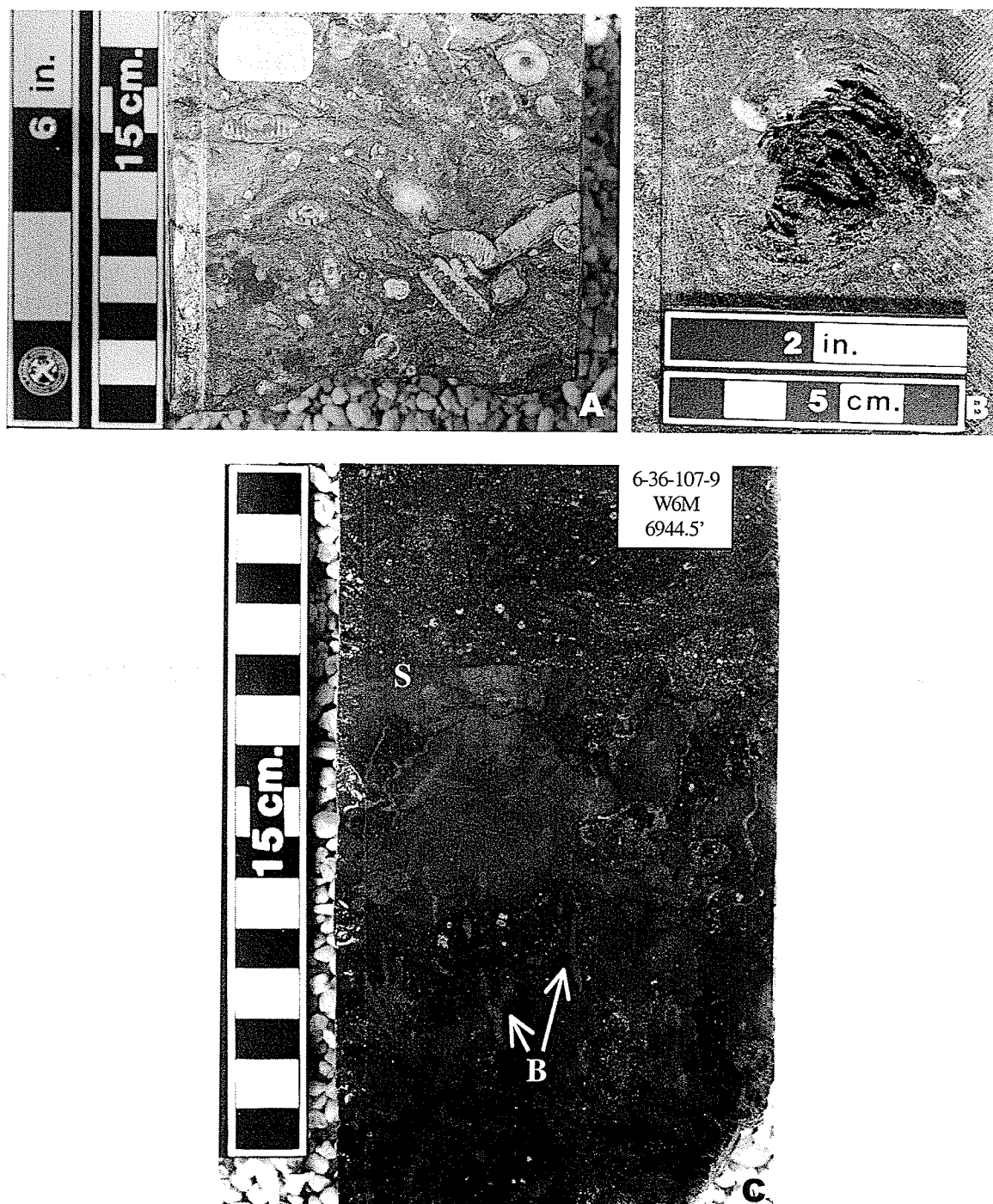
Figure 3.8 Core photographs of Lithofacies E: bioturbated crinoid-brachiopod floatstone. A) Crinoid floatstone to rudstone showing large articulated ossicles. 4-19-116-4 W6M, 1564.8 m (5134 ft). B) Brachiopod-crinoid-stromatoporoid floatstone exhibiting biomoldic porosity created by leaching of a nodular stromatoporoid. 4-16-108-8 W6M, 1987.9 m (6522 ft). C) Pervasively bioturbated crinoid-brachiopod wackestone displaying well-defined vertical burrows (B) and scour surface (S). 6-36-107-9 W6M, 2116.7 m (6944.5 ft).
