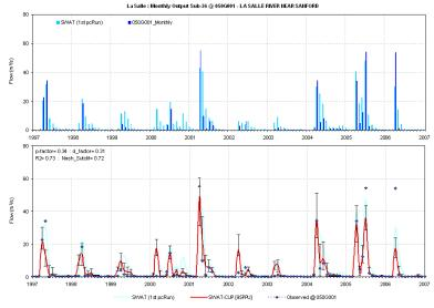
**Figure 5.** Monthly SWAT output calibration with GLUE from SWAT-CUP (top: daily flows and nutrients with 1<sup>st</sup> set of parameters; bottom: monthly values-95% uncertainty brackets)
