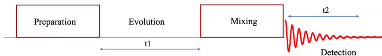
Figure 31. Scheme of a typical two-dimensional NMR experiment with all four parts outlined.
