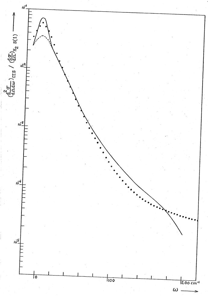
Comparison of the Experimental and Calculated DID CIS Spectrum for  $\mathrm{CF}_{l_{\!\!\!\! +}}$
