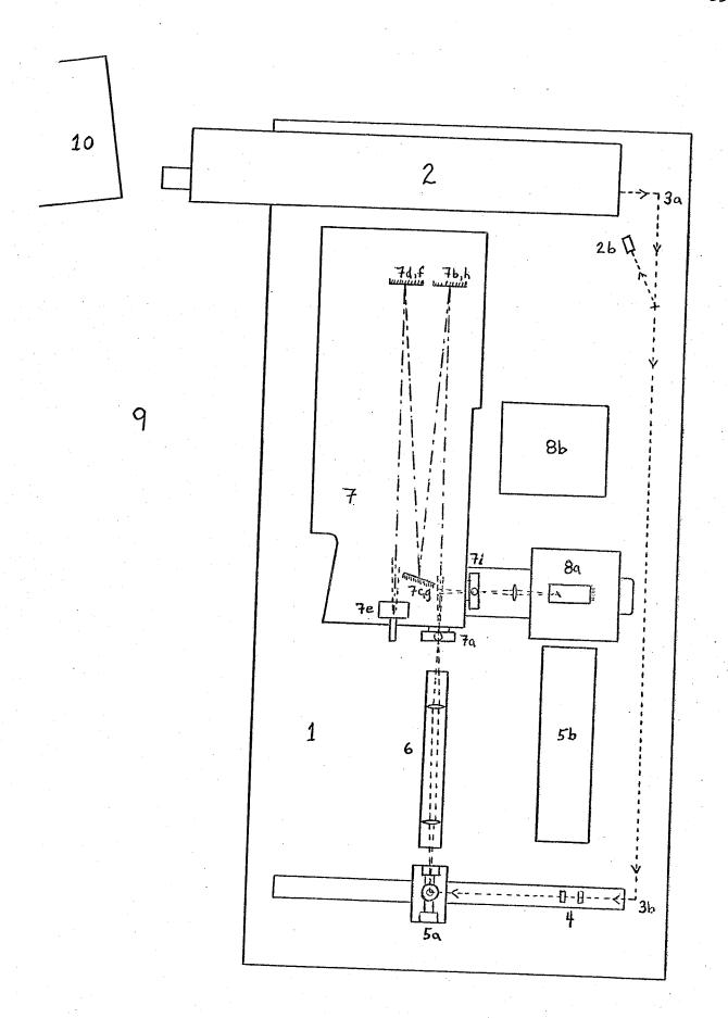
anti-reflection coated, the intensity of the beam is only one half of its original value by the time the beam has entered the sample — the sample is typically illuminated by a power of 300 mW or  $7.5 \times 10^{17}$  photons/sec at a wavelength of 4880 Å.
