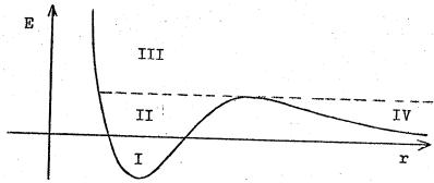
Particles in region I, with total energy E < 0 will be bound. Particles in region II, with total energy less than the local maximum, will remain bound so long as L is left unchanged — they may be called metastably bound. Particles in region IV have the same energy as particles in region II, but started to the right of the local maximum — we may call them low energy free particles. The remainder, region III, is composed of high energy free particles.
