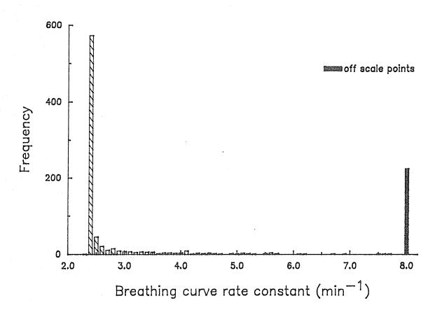
The distribution of grey matter flow estimates corresponding to the distribution of the breathing curve rate constant b shown in figure 12. The input flow value was 0.8 ml/ml/min
