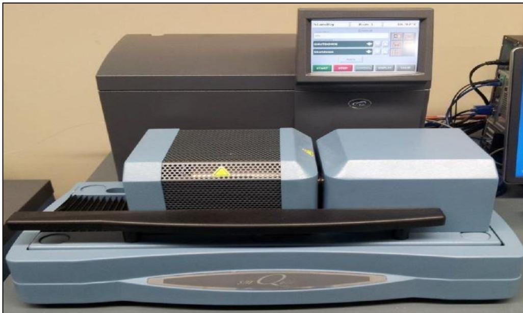
**Figure 3.9** Differential Scanning Calorimetry (DSC) apparatus.
