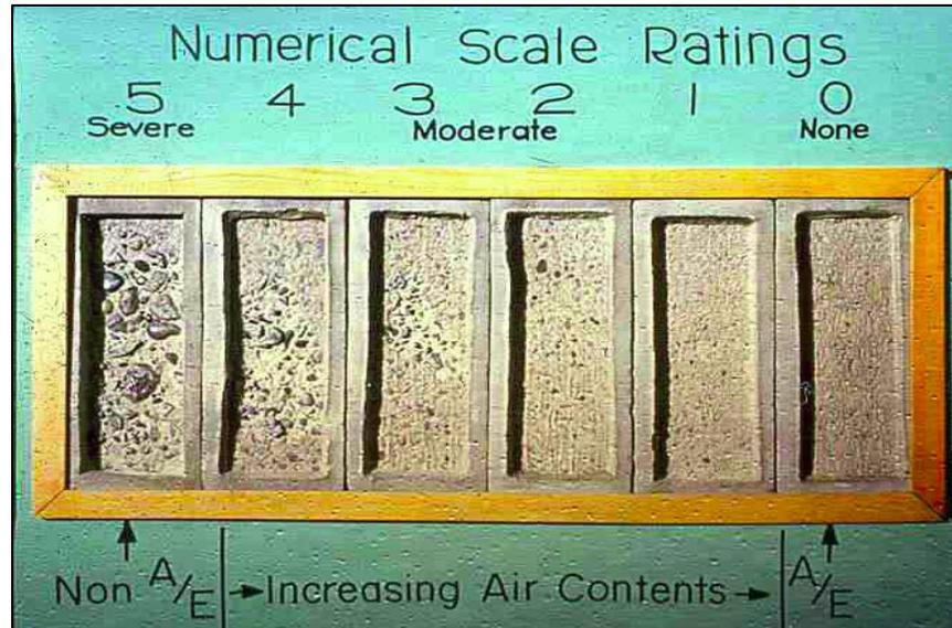
**Figure 3.12** Visual rating of concrete surface scaling.
