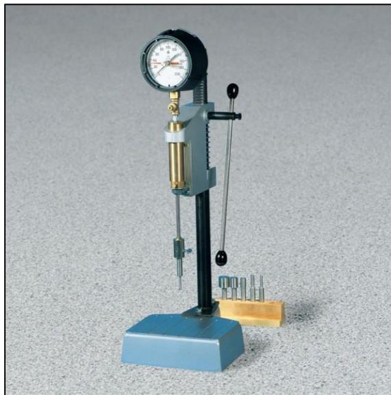
**Figure 3.7** ACME penetrometer setting time apparatus.
