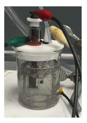
**Figure 1.11.** Bulk Electrolysis setup used in this work. Ar/CO<sub>2</sub> is bubbled into solution, with the solution stirred in the working electrode compartment (Pt mesh electrode shown) where the reference electrode (white electrode) is placed. The counter electrode (graphite rod) is placed in a separate glass-tube, connected to the working electrode solution through a frit to prevent product crossover.
