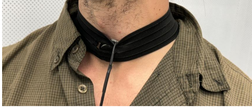
Fig. 6-2: Subject position and microphone placement for Tracheal breathing sounds recording (Test 2).
