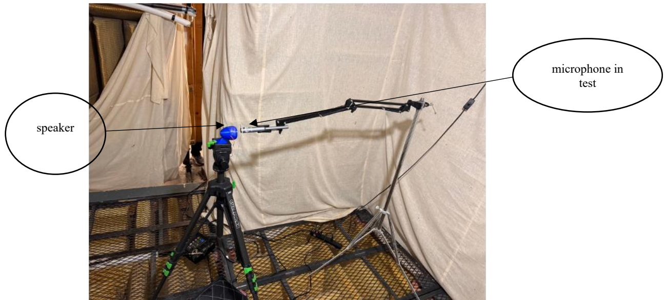
Fig. 6-1: Test 1 setup in the anechoic chamber.
