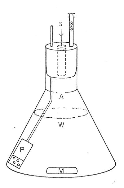
The apparatus was placed back into the  $20 \pm 1^{\circ} \text{C}$  water bath in which the water level reached the top of the rubber stopper but did not flood the septum cap area, thereby preventing contamination of gas samples with water. The magnetic stirrer was engaged and  $0_2$  decrease in the air was determined using gas chromatograph samples drawn periodically through the septum, while  $0_2$  decrease in the water was monitored using the YSI oxygen meter and strip chart recorder.
