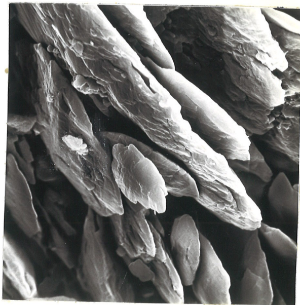
Figure 43. SEM photograph of concretion-like aggregates and acicular crystals of thenardite (Apks "Rego Black, saline phase").
