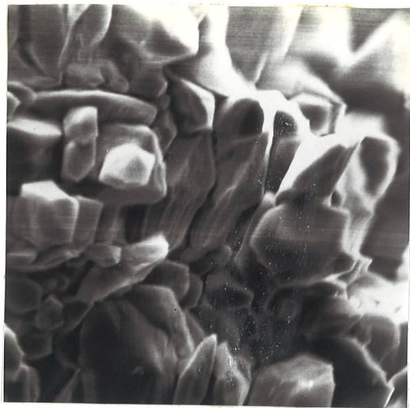
Figure 42. SEM photograph of prismatic and closely packed features in agypsiferous material (Ahs "Gleyed Calcareous Black, saline phase").
