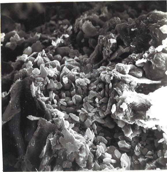
Figure 40. SEM photograph of lenticular-hexagonal gypsum microlites (AC "Rego Black, saline phase").
