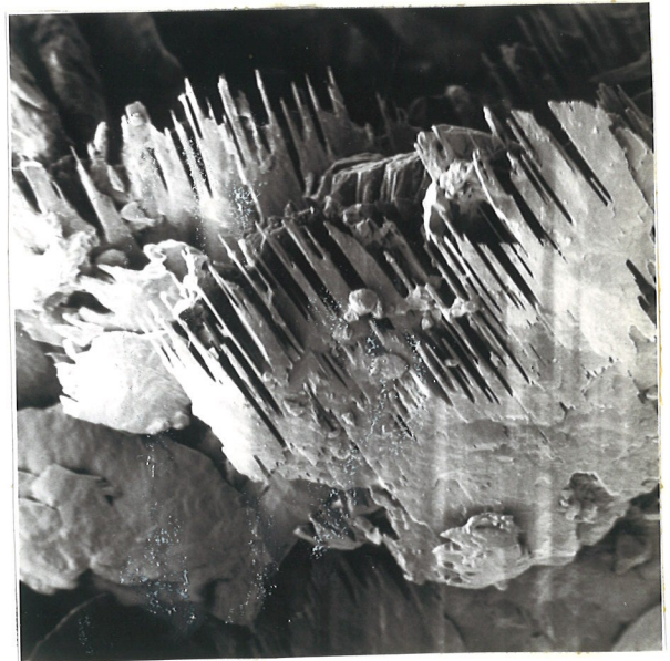
Figure 41. SEM photograph of cave like with comb-structure in weathered gypsiferous material (AC "Rego Black, saline phase").
