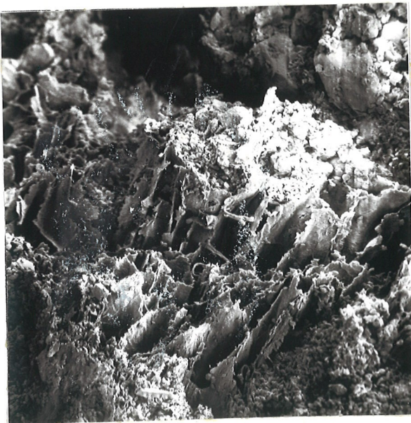
Figure 41. SEM photograph of cave like with comb-structure in weathered gypsiferous material (AC "Rego Black, saline phase").
