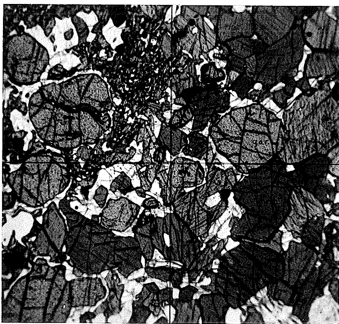
B - Photomicrograph of hornblende-garnet rock. Plagioclase surrounds garnet grains, and is intergrown with clinopyroxene. Plane polarized light, magnification 180x.
