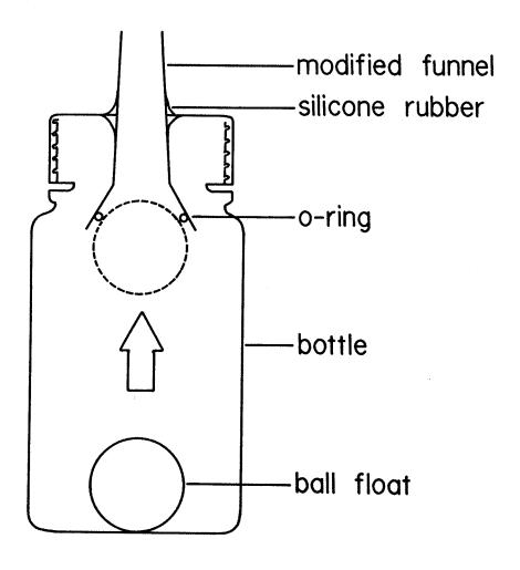
nent stake at each sampling station with wide rubber bands to facilitate removal of samples. In most cases, rubber bands were replaced every two weeks because of saltwater corrosion. During sampling, the cap was removed and the ball float removed from filled bottles with forceps, and placed in a new clean bottle. The cap was secured and the new bottle was attached to the stake.
