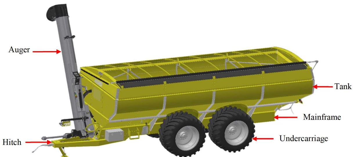
Figure 2. Elmer's Manufacturing Inventor model of the HaulMaster 2500 grain cart [9].
