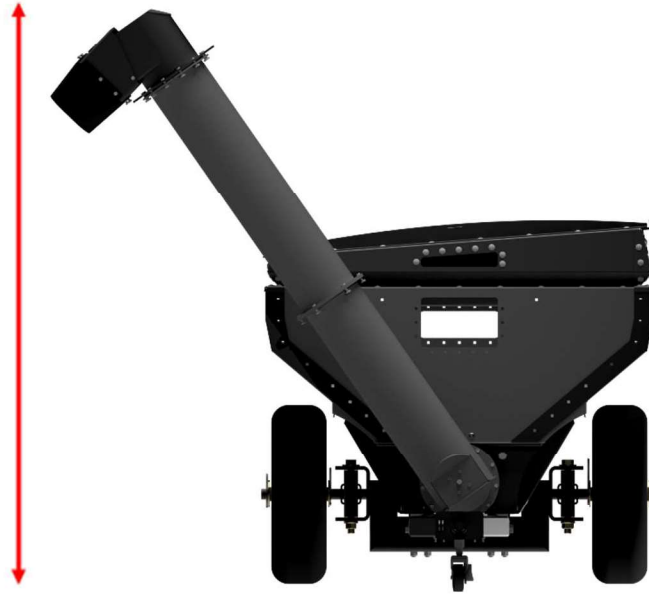
Figure 27. Height verification of the grain cart with auger mounted.
