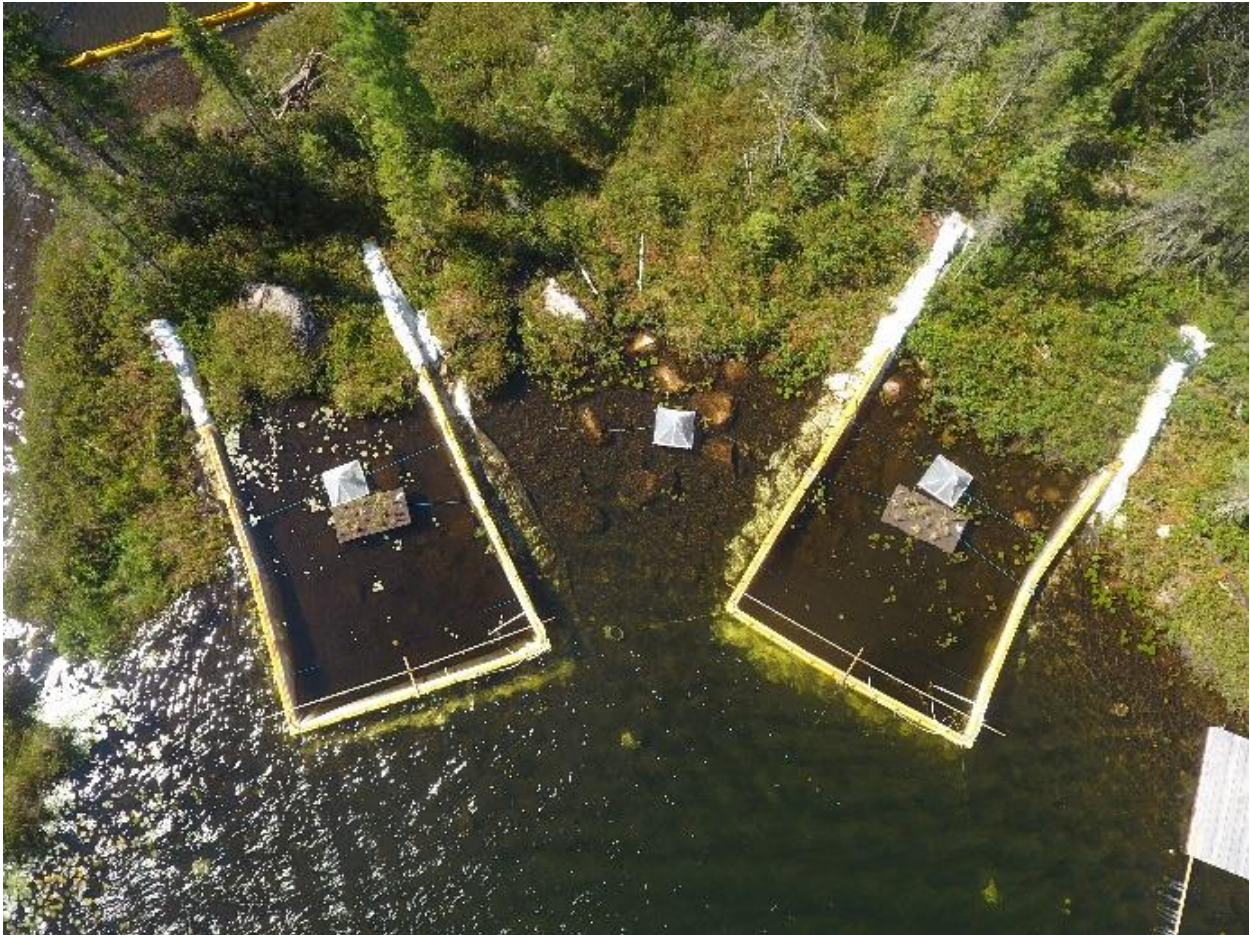
Figure B1. Drone image of the FLOWTER 2021 shoreline enclosures (Curry Industries Ltd, Winnipeg) with deployed EFWs on Lake 260 at the IISD Experimental Lakes Area. LR EFW is to the right (west) of the photo. Source: IISD-ELA.
