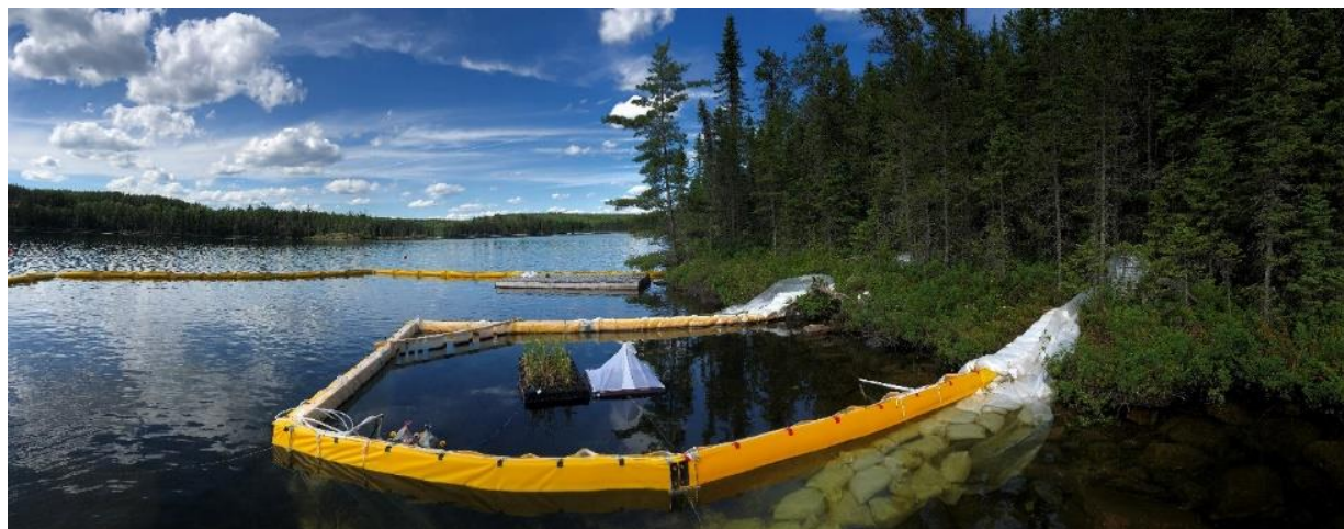
Figure A1. Example of a shoreline enclosure (Curry Industries Ltd., Winnipeg) in a rock cobble environment highlighting the floating collar attached to a polypropylene curtain sealed to the sediment and onto the shoreline, and EFW and sampling equipment.
