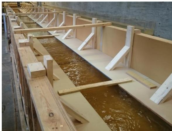
**Figure 3-2: Installed border ice.**
