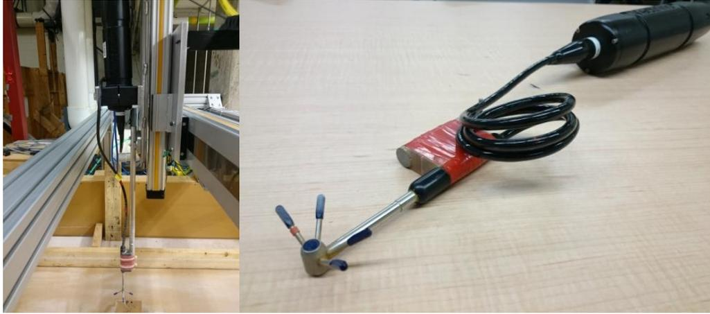
**Figure 3-3: Vectrino II Profiling ADV (left) and Vectrino + ADV (right).**
