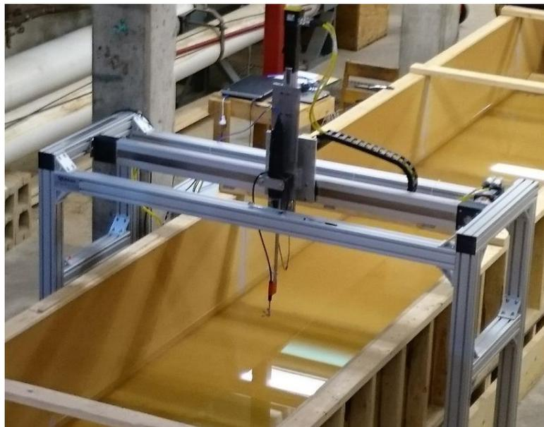
**Figure 3-5: Traversing Mechanism**
