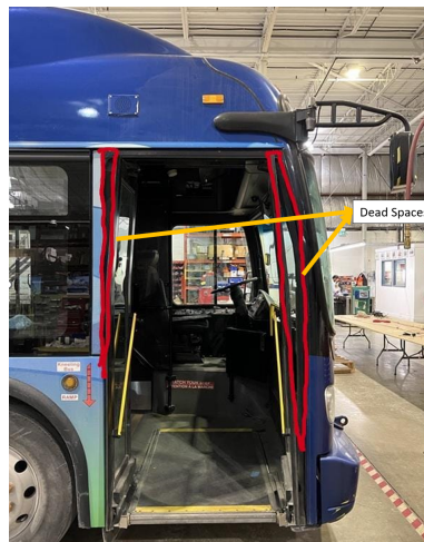
Figure 1: Dead space areas highlighted on entrance door.
