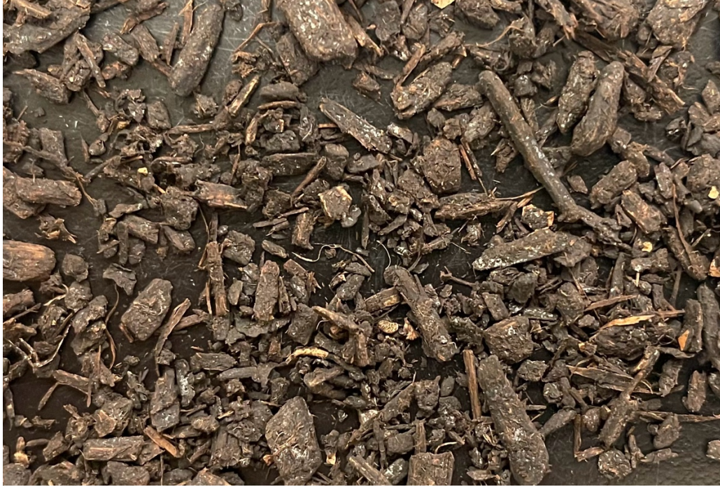
Figure 3.2 Compost recovered from thermophilic respirometer vessels (58 °C) following complete PLA mineralization. White deposits on wood chip surfaces were observed equally across all conditions, including negative controls without PLA, and are attributed to mineral precipitates.
