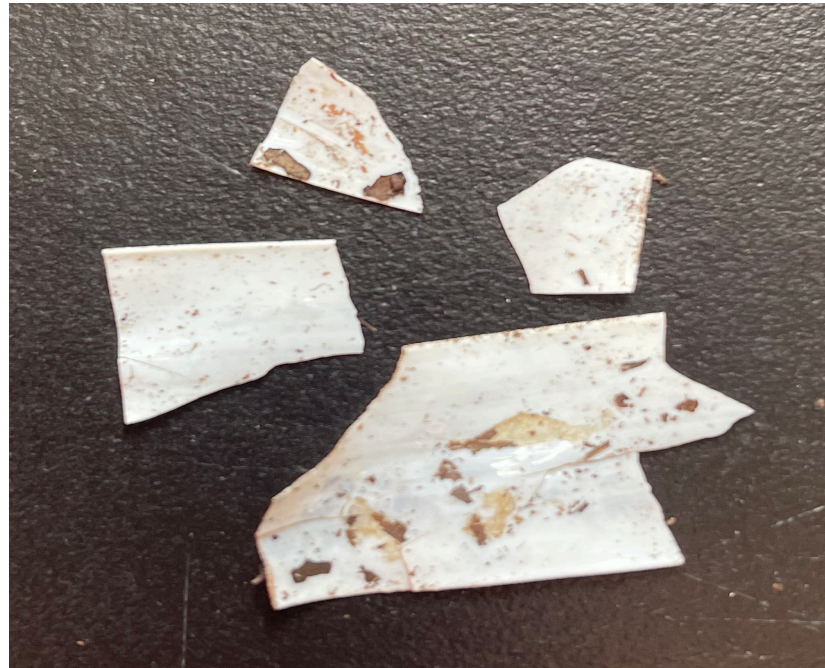
Figure A1 – Lightly fragmented PLA film with 100% recovery
