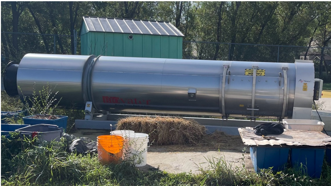
Figure 4.3 Exterior view of the SIAF RDC (Winnipeg, MB), an 18-foot rotating in-vessel composting unit used in experiments.
