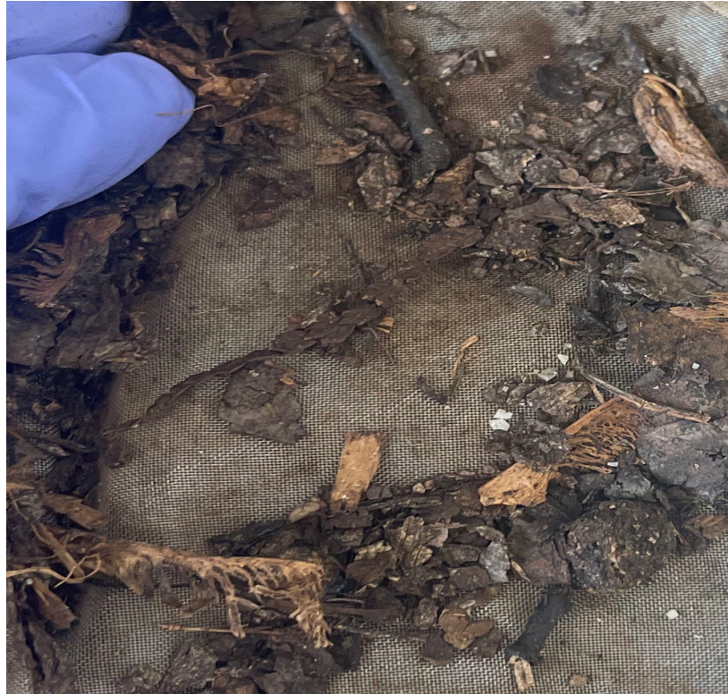
Figure A2 – Heavily fragmented/powderized PLA film with 22% recovery
