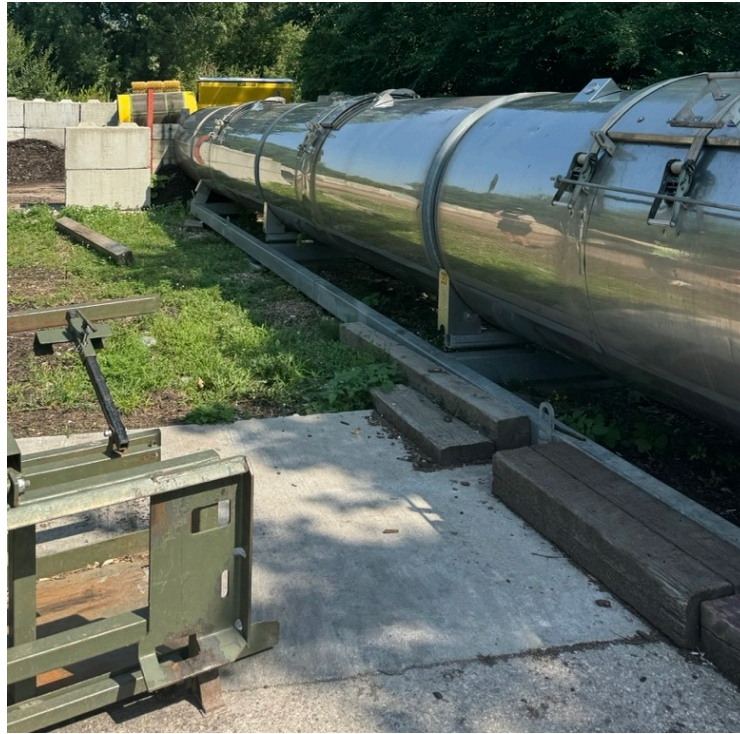
Figure 4.4 Exterior view of the Forks Market RDC (Winnipeg, MB), a 42-foot rotating in-vessel composting unit used in experiments.
