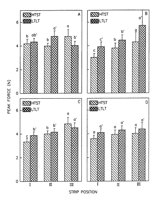
Figure 14. Effect of strip position on peak deformation of french fry strips for two different blanching methods (n = 5). Error bars are ±95% CL. A - Shilo (1994); B - Shilo (1995); C - Portage (1994); D - Portage (1995). HTST means followed by different letters (eg. a) are significantly different from each other (p≤0.05). LTLT means followed by a different letter followed by prime symbol (eg. a') differ significantly from each other (p≤0.05).
