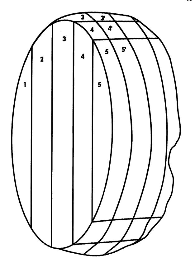
4', 5 and 5' from the same half-tuber were used for colour measurements. Strips 3' and 2' (2' not shown in Figure but is behind strip 2) were used for moisture content determinations. Strip 1' was not used. Only those strips used for measurements of mechanical properties were marked prior to processing.
