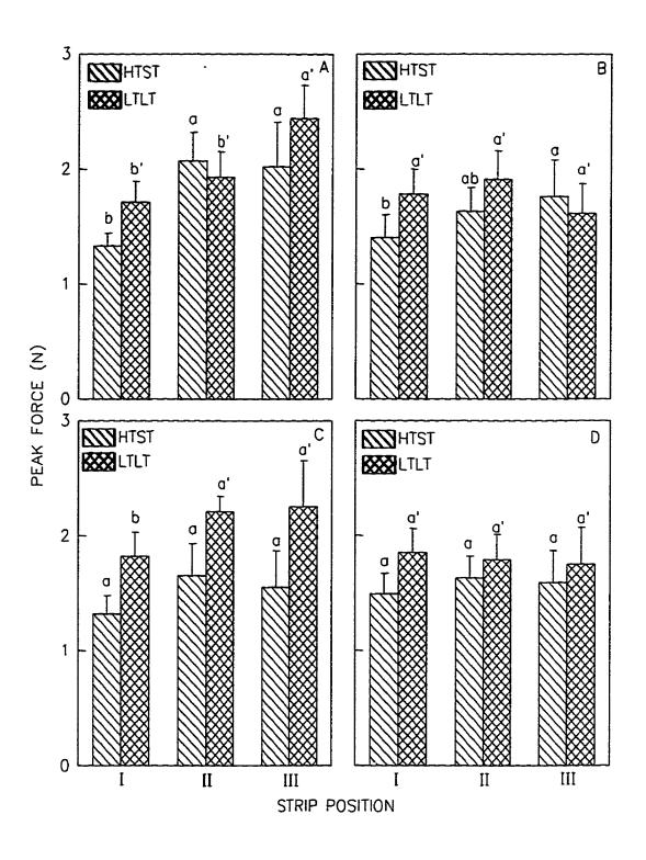
Figure 17. Effect of strip position on peak deformation of french fry strips for two different blanching methods followed by freezing (n=5). Error bars are ±95% CL. A - Shilo (1994); B - Shilo (1995); C - Portage (1994); D - Portage (1995). HTST means followed by a different letter (eg. a) differ significantly from each other (p≤0.05). LTLT means followed by a different letter followed by prime symbol (eg. a') are significantly different from each other (p≤0.05).
