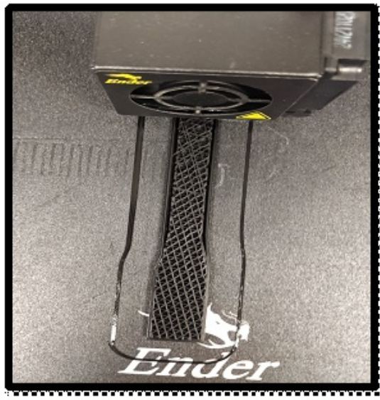
Figure 3.5: Tensile Specimen printing in 3D printer.
