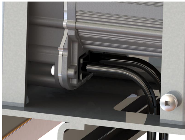
Figure 43: Tilt motor cable routing.
