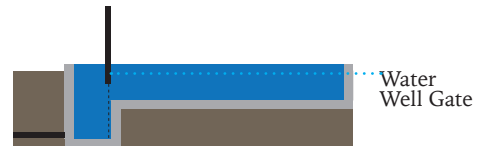
Section of water canal
