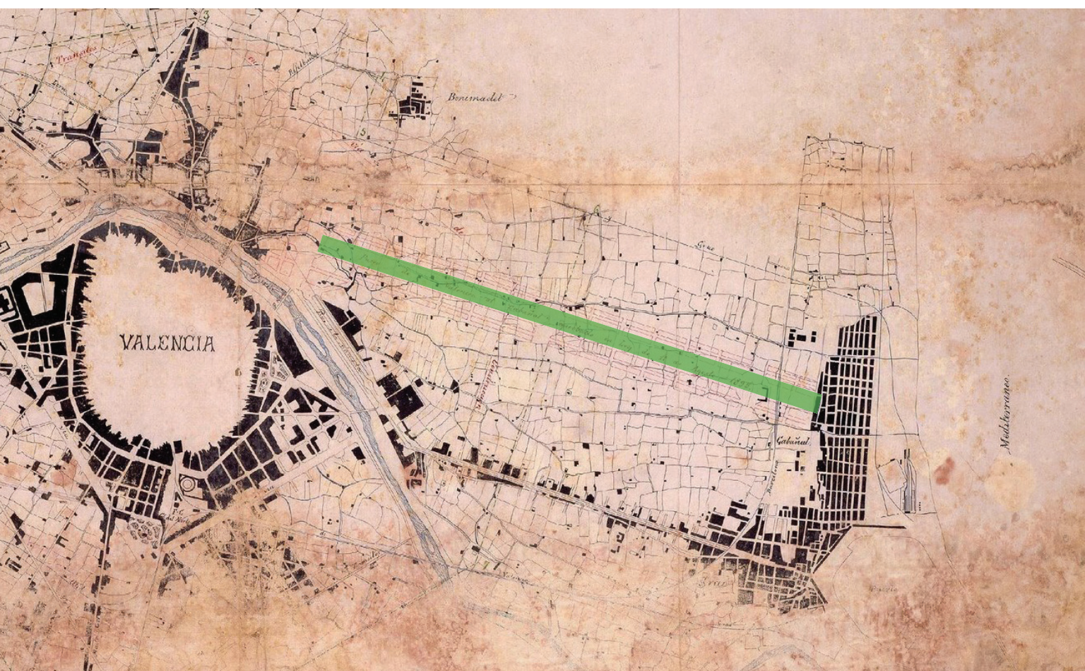
FIG. 13. Plan "Paseo Valencia al Cabanyal". Highlighted green is the 100m wide boulevard that would bisect the barri.
