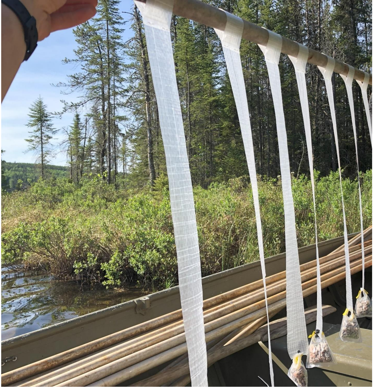
Figure 2.5: The polypropylene strips used for sampling biofilm during the FOReST project. (Photo credit: Madeline Stanley).
