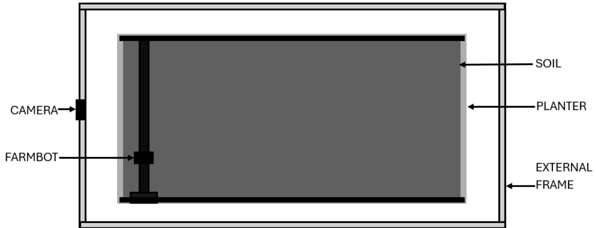
Figure 2: Top view of the planter workspace of the FarmBot during experimental sessions
