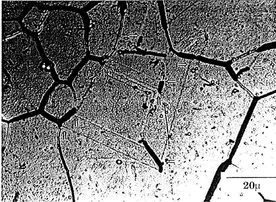
Figure 2.5.3 Optical micrograph with arrows indicating intergranular attack being resisted at twin boundaries in processed material [50].
