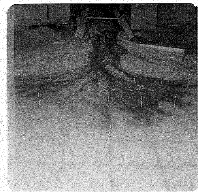
CHANNEL BRAIDING AT Q = 0.020 cfs, T = 60 MIN.
