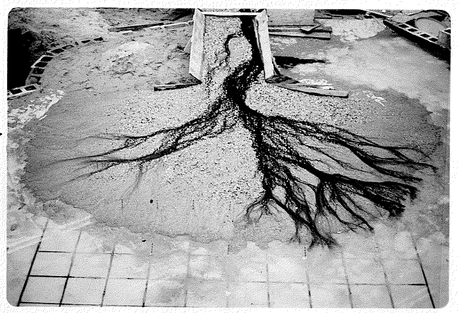
CHANNEL SHIFTING AT Q = 0.020 CFS, T = 60 MIN.
