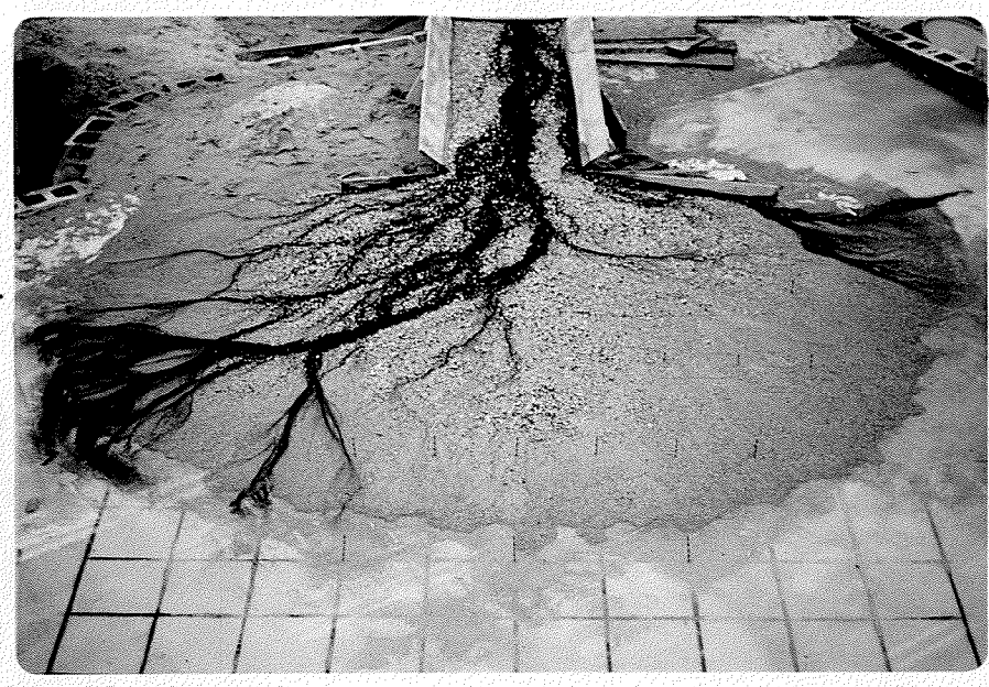
INCREASED CHANNEL BRAIDING AT Q = 0.010 CFS, T = 50 MIN.
