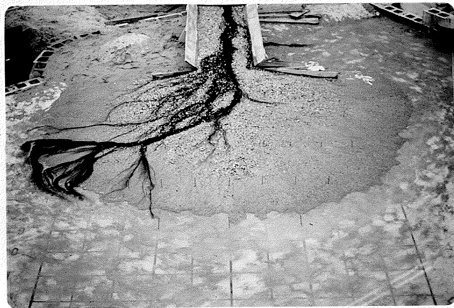
CHANNEL LOCATION AT Q = 0.005 cfs, T = 40 MIN.
