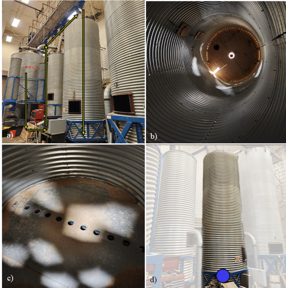
Figure 3.7: Experimental silo setup for pressure measurements. a) Material flow path showing grain transfer from main storage silo through elevator system to the instrumented test silo; b) Interior view looking upward at the silo inlet where grain enters from the elevator; c) Empty silo floor showing multiple radial discharge points (holes) that can be individually opened and closed to control the grain flow pattern during emptying; d) Exterior view of the test silo with sensor location marked (blue circle) where triaxial pressure measurements were taken.
