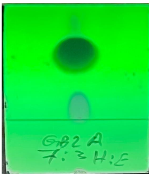
Figure 5. Thin-layer chromatography (TLC) analysis of a fraction derived from the GB2 crude extract developed using a hexane:ethyl acetate (7:3, v/v) solvent system. Differences in band number and migration distance reflect variation in compound polarity among the detected metabolites.
