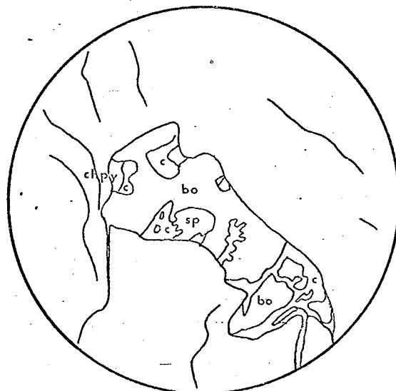
(d) An exsolved 'bleb' in pyrite contains bornite, chalcocite, chalcopyrite and sphalerite (1360X).
