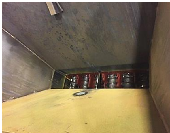
Figure 4. Top view of the hopper from Ultra-Span's concrete extruder [1]
