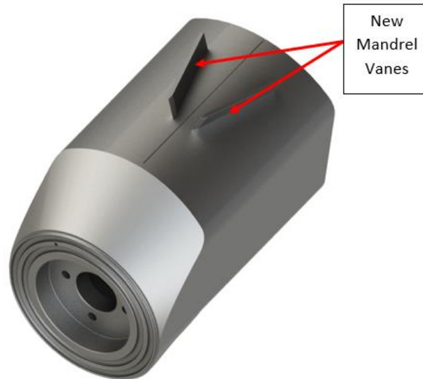
Figure 16. Concept H: Mandrel Vanes (isometric view)
