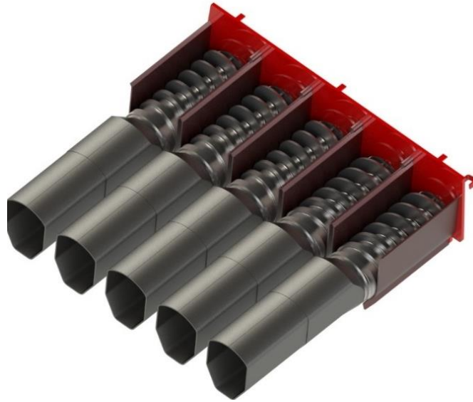
Figure 14. Concept D: Sealed and Elongated Material Shields (isometric view)
