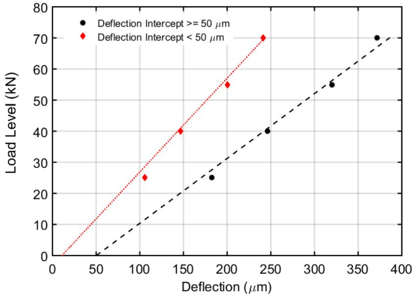
Figure 2-20: Crovetti's Void Detection Procedure Using FWD Data
