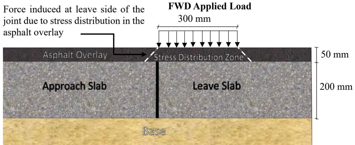
Figure 4-9: Stress Distribution Across Asphalt Overlay Causing Overestimated Joint Performance.
