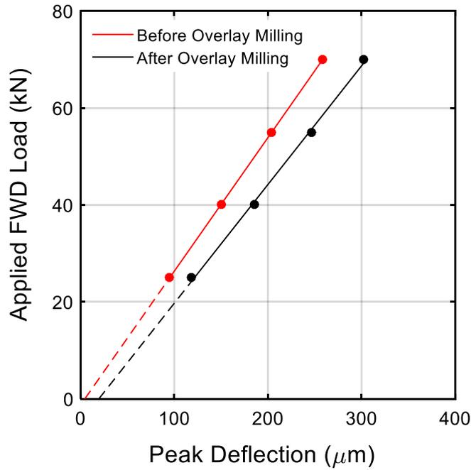
Figure 4-13: Joint Deflection-Load Plot Before and After Milling.
