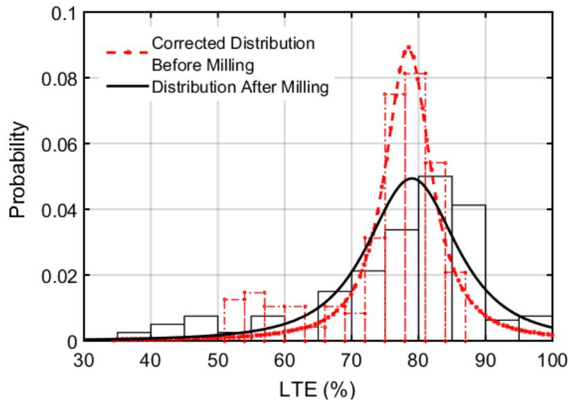
Figure 4-19: Probability Distribution of Corrected LTE Before Milling and After Milling.
