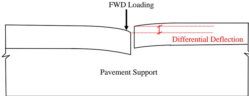
Figure 2-13: Illustration of Differential Deflection in Concrete Pavements.
