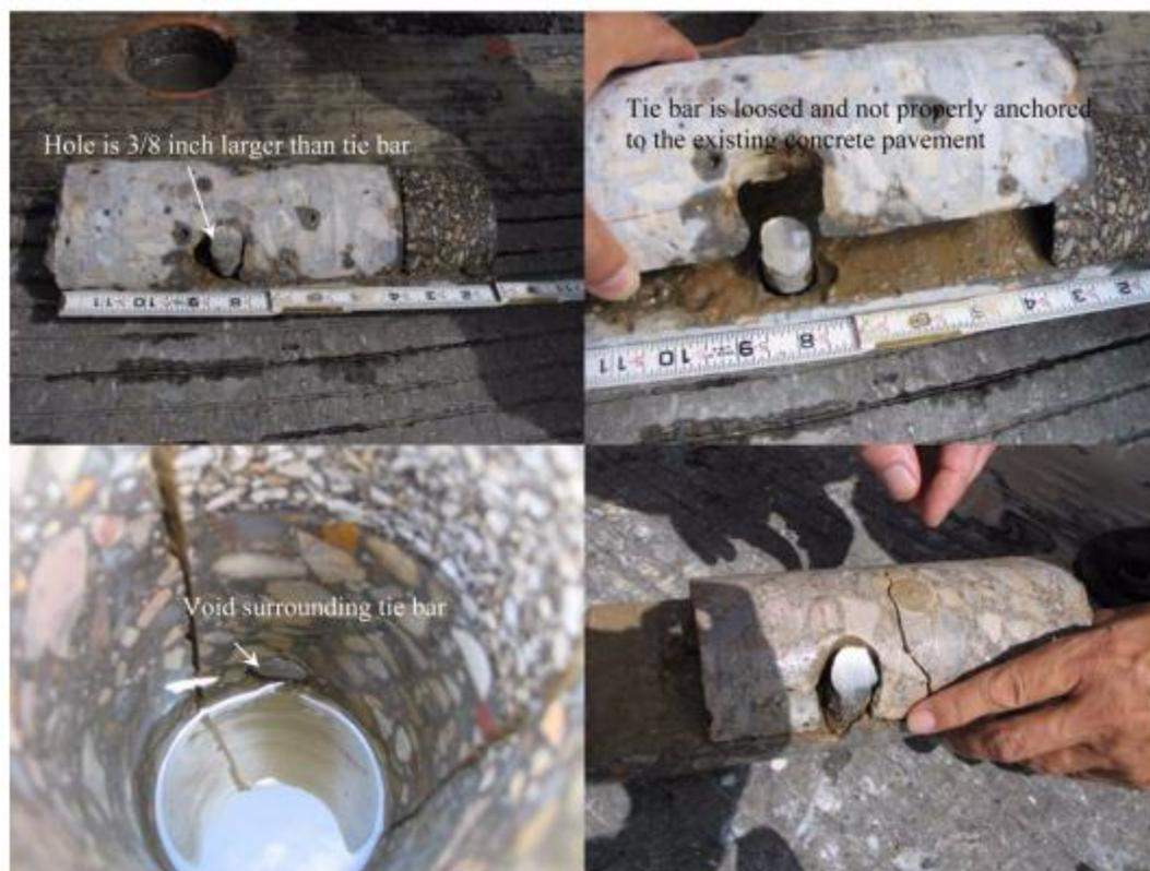
Figure 2-2: Tie Bars Deterioration in PCC Joints (Chen, Hong, et al., 2011).
