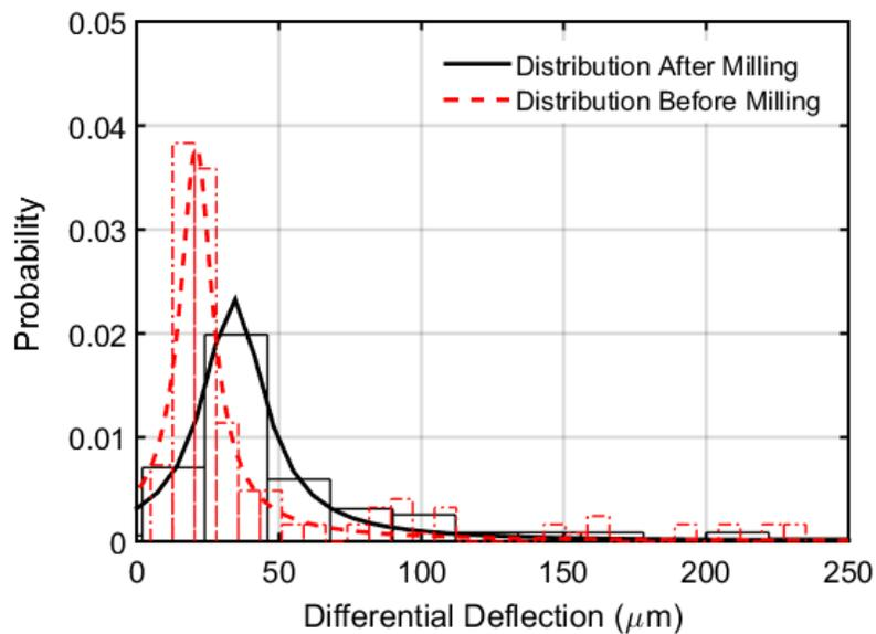
Figure 4-11: Probability Distribution of Differential Deflections Before and After Milling.
