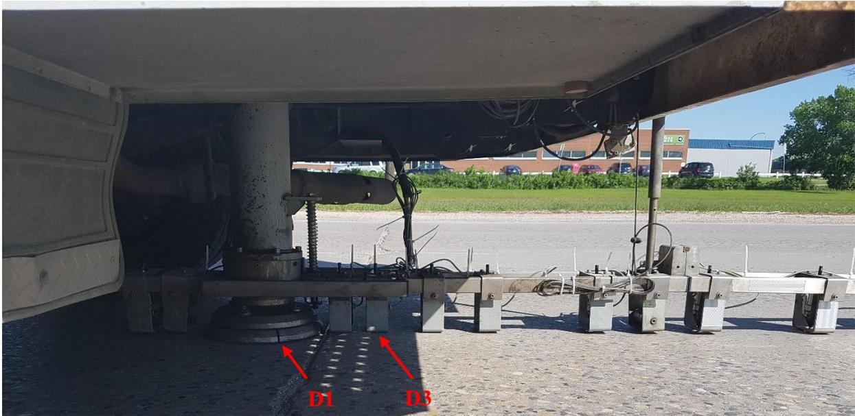
Figure 3-6: Leave Joint FWD Testing on Concrete Pavement of McGillivray Boulevard.
