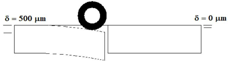
Figure 2-15: Schematic of Low LTE and High Differential Deflection.
