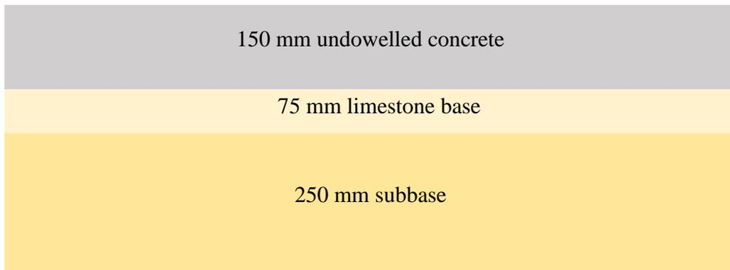
Figure 3-2: Typical Residential Street Pavement Structure.
