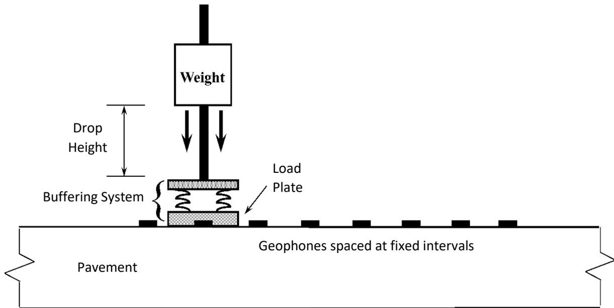
Figure 2-7: FWD Testing System Schematic (Smith et al., 2017).
