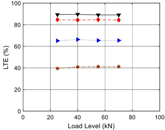
Figure 4-7: LTEs Variation with Load Levels.
