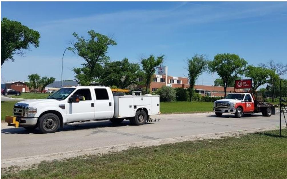
Figure 3-4: Falling Weight Deflectometer with RTK Survey Equipment.
