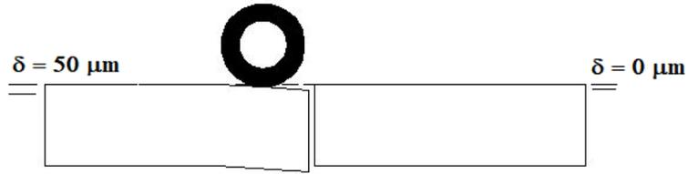
Figure 2-14: Schematic of Low LTE and Low Differential Deflection.
