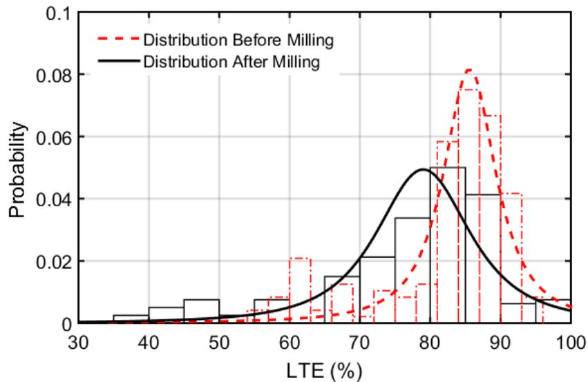
Figure 4-12: Probability Distribution of LTEs Before and After Milling.
