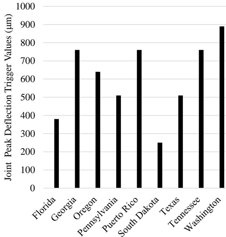
Figure 2-18: Peak Deflection Trigger Value in Different States.
