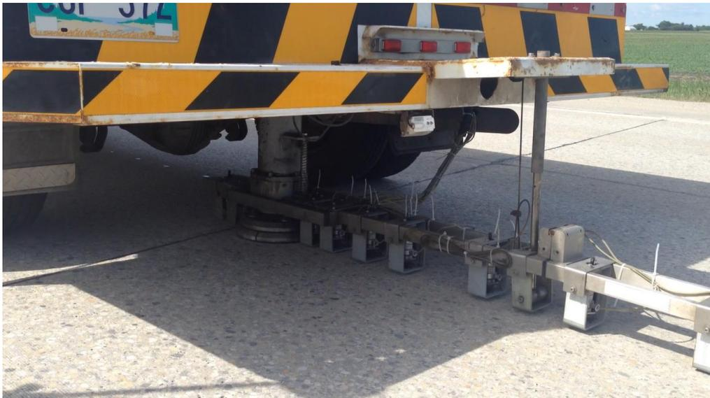
Figure 2-8: Falling Weight Deflectometer Load Plate and Deflection Geophones.
