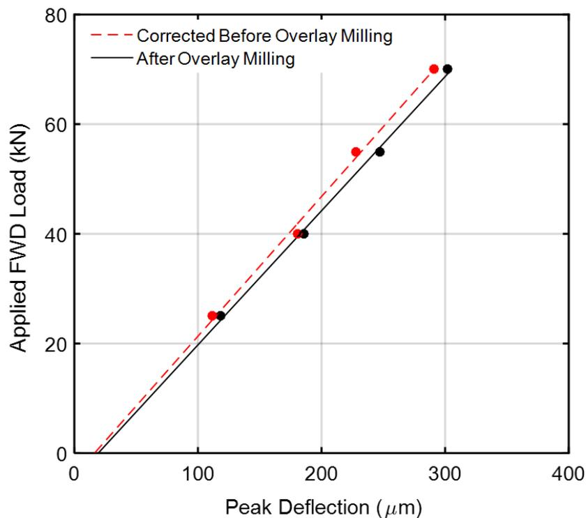
Figure 4-20: Corrected Joint Deflection-Load Plot Before and After Milling.
