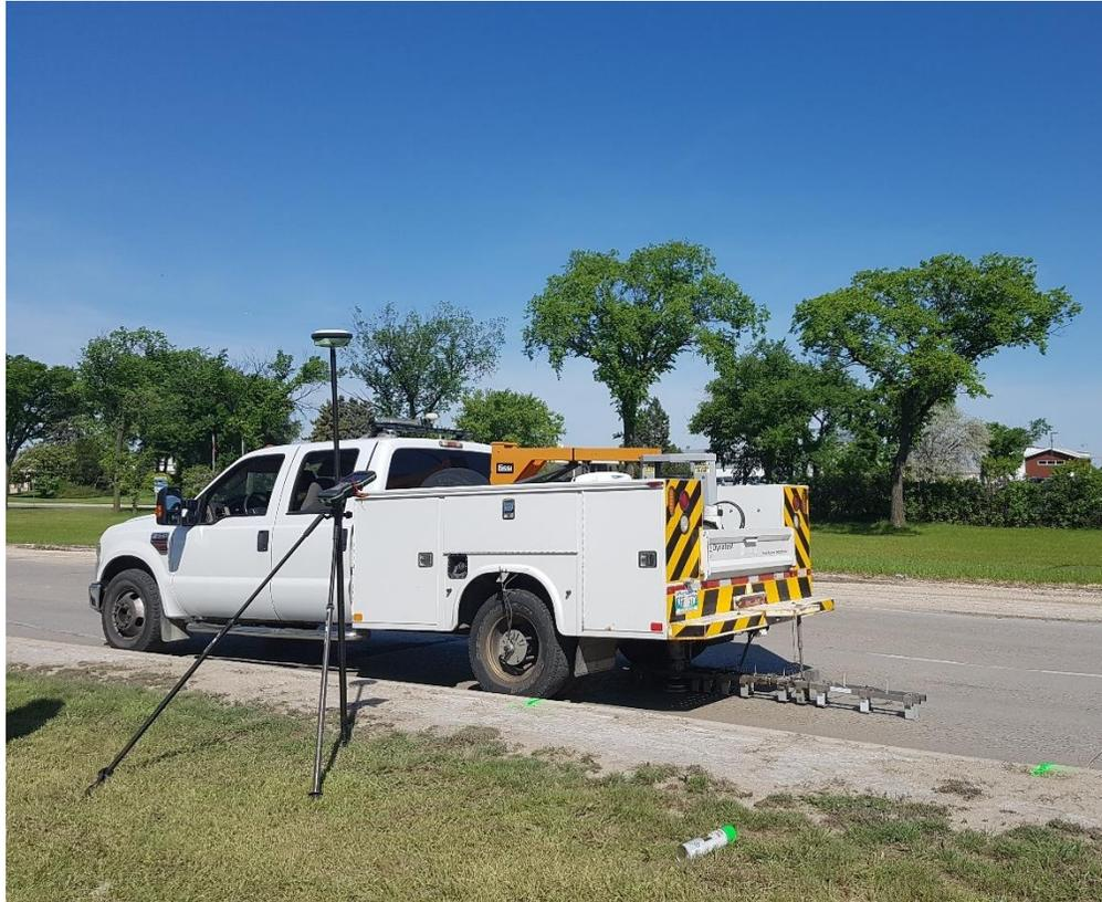
Figure 2-6: Dynatest Falling Weight Deflectometer.
