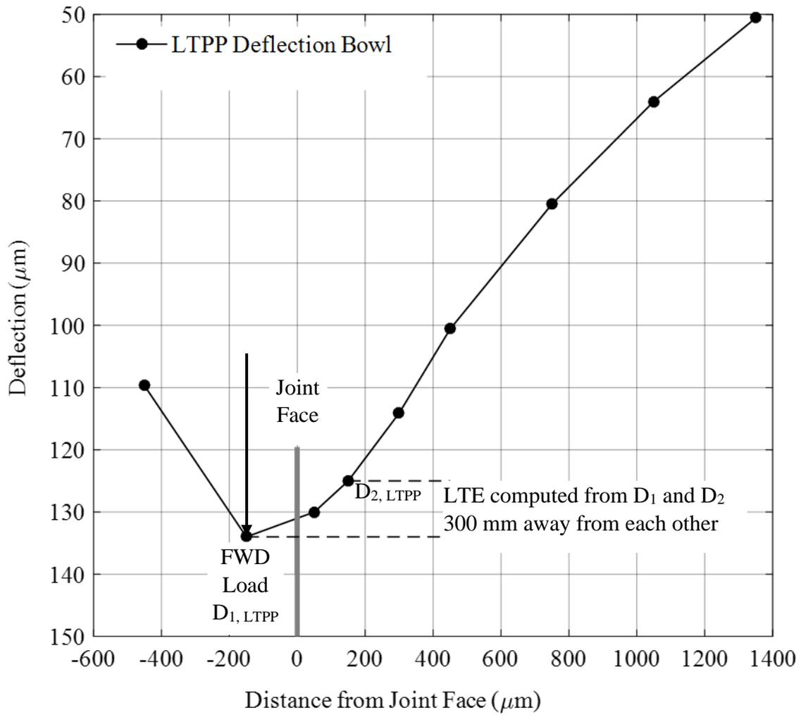
Figure 4-3: LTPP Layout Deflection Bowl at Joint.
