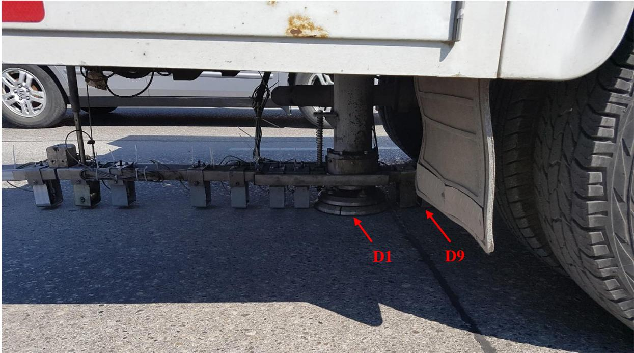
Figure 3-5: Approach Joint FWD Testing on Asphalt Overlay of Pembina Highway.
