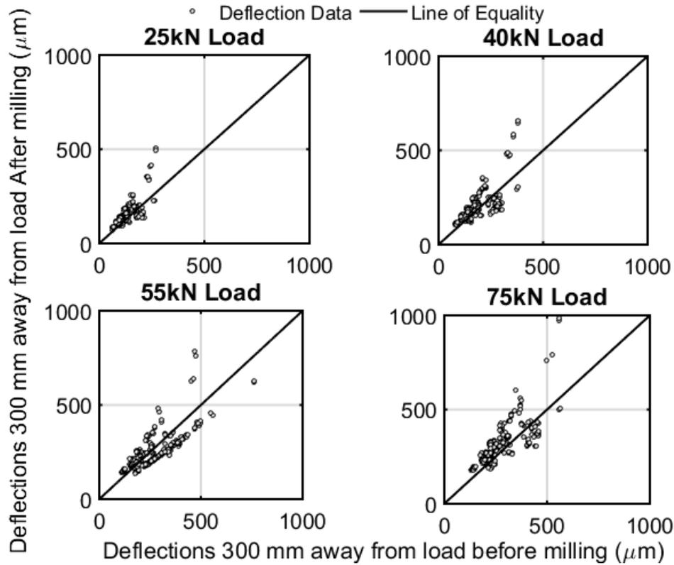
Figure 4-16: Relationship between Deflections 300 mm Away from Load Plate Before and After Milling at Different Loads.
