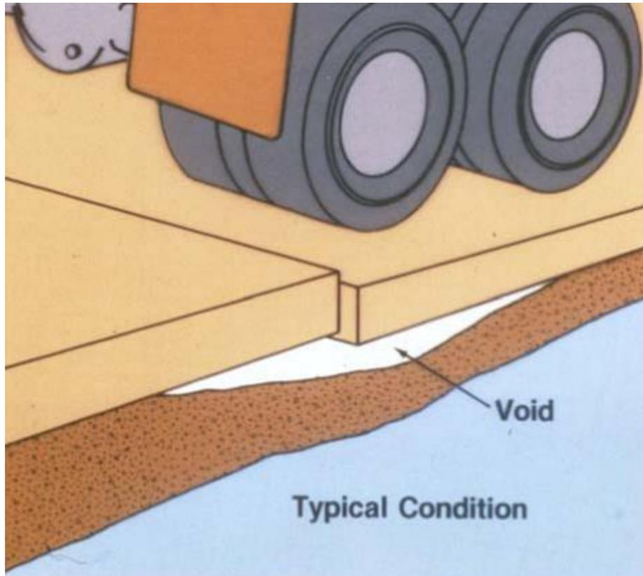
Figure 2-5: Development of Void under Joints (Stahl, 2006).
