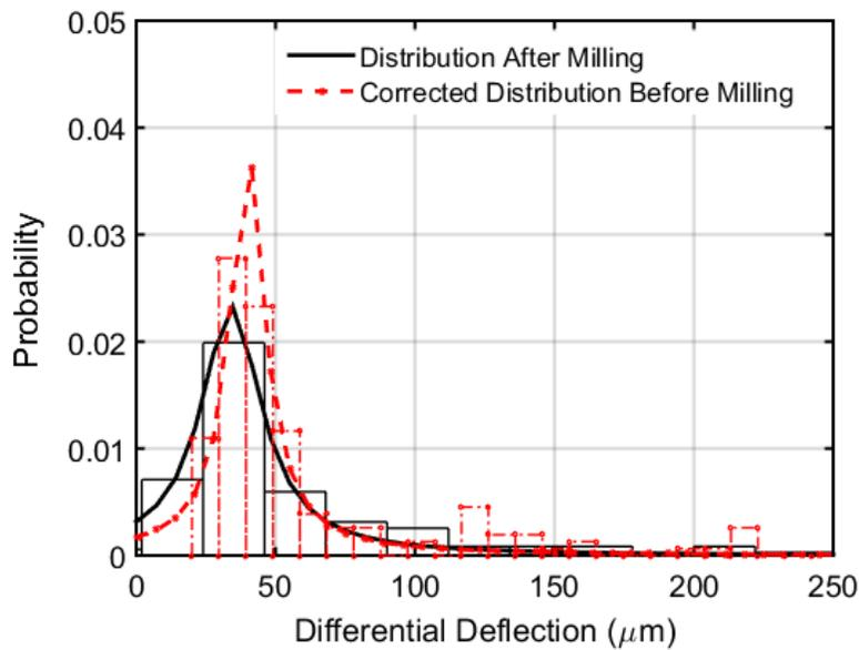
Figure 4-18: Probability Distribution of Corrected Differential Deflections Before Milling and Differential Deflections After Milling.
