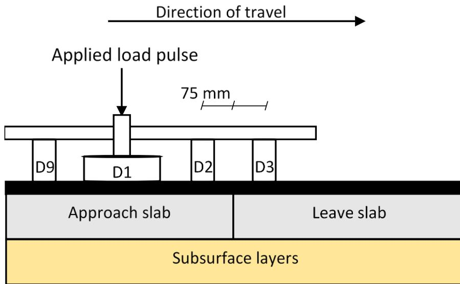
Figure 2-19: FWD Geophones Layout for Composite Joint Testing (Strata Engineering Corporation, 1998).
