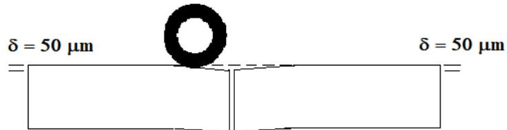
Figure 2-16: Schematic of High LTE and Low Differential Deflection.
