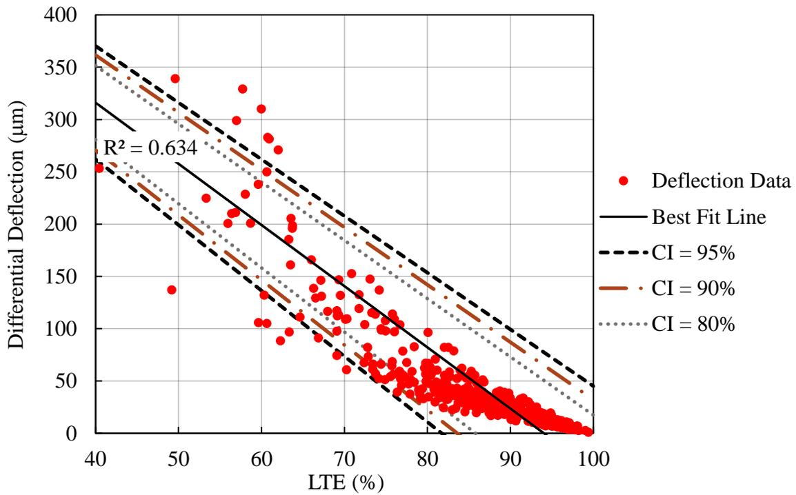
Figure 4-5: Relationship between Load Transfer Efficiency and Peak and Differential Deflections.
