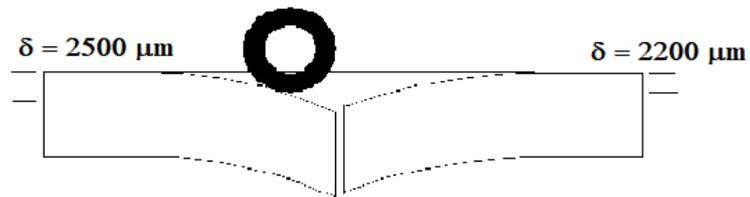
Figure 2-17: Schematic of High LTE and High Differential Deflection.
