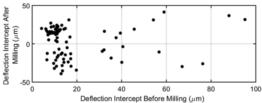
Figure 4-14: Void Detection Analysis Using Deflections Before and After Milling.
