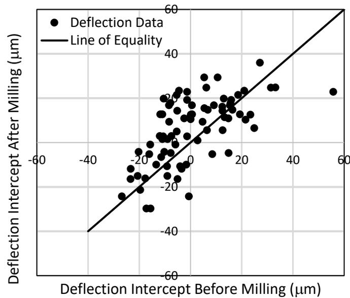
Figure 4-21: Comparison of Void Detection Analysis Results from Corrected Pre-Milling Deflections and Post-Milling Deflections.
