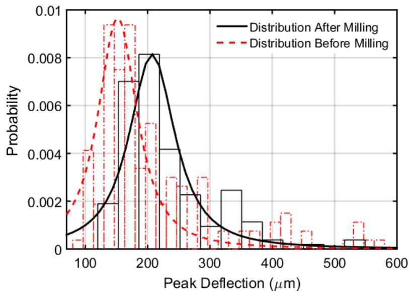
Figure 4-10: Probability Distribution of Peak Deflections Before and After Milling.
