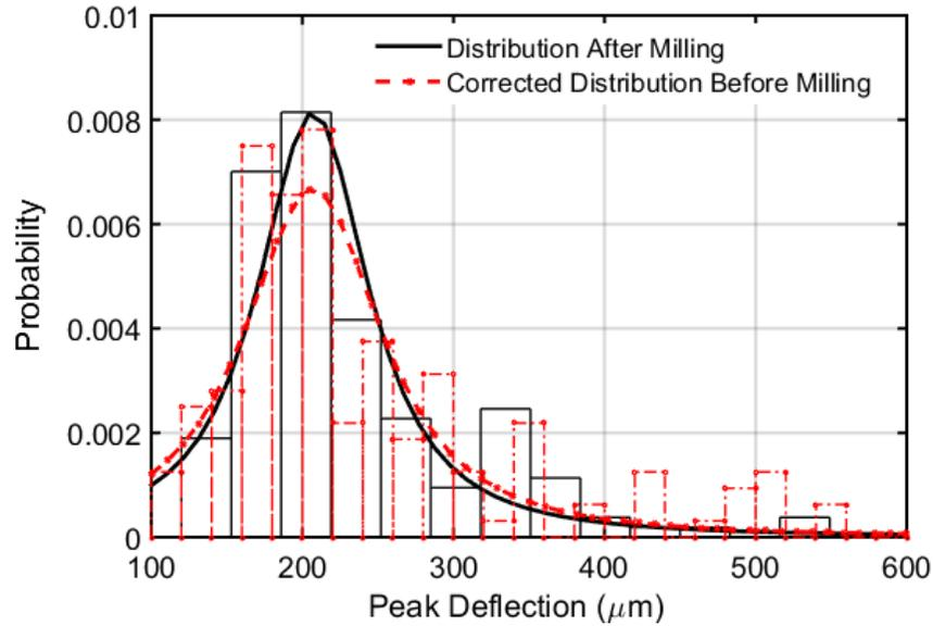
Figure 4-17: Probability Distribution of Corrected Peak Deflections Before Milling and Peak Deflections After Milling.
