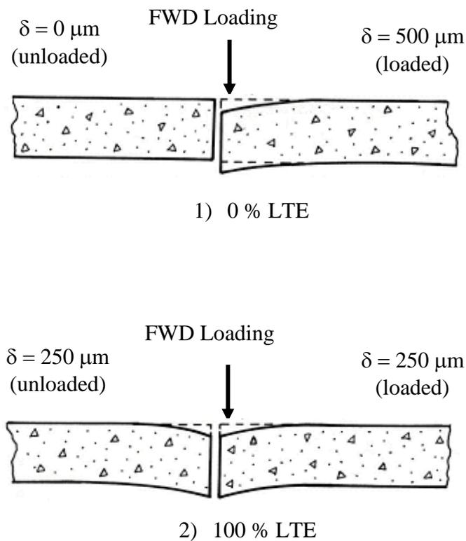
Figure 2-9: Comparison of a) 0 % and b) 100% LTE.
