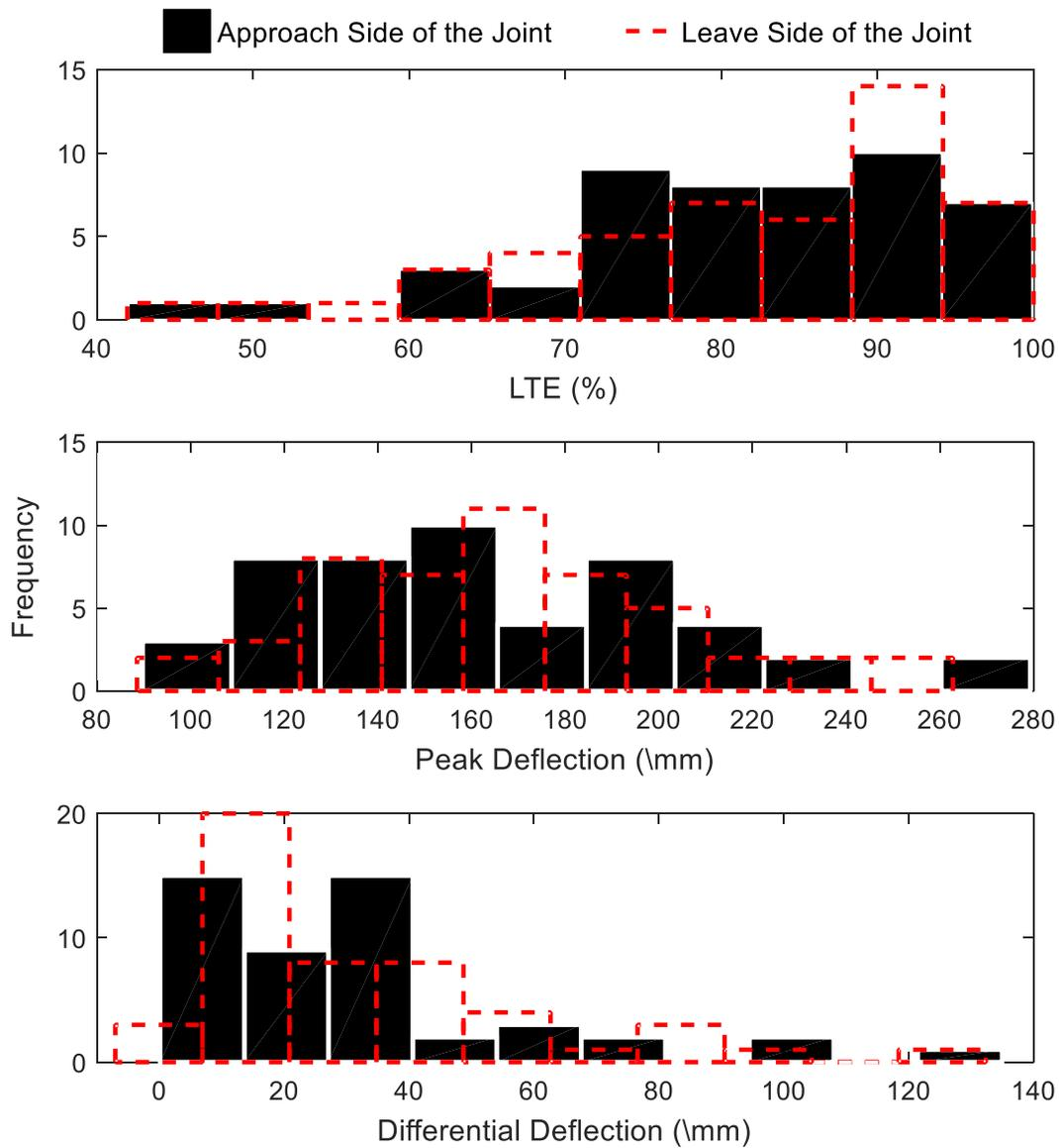
Figure 5-1: Histograms of Load Transfer Efficiency, Peak Deflection, and Differential Deflection of Joints After Full-Depth Repair.
