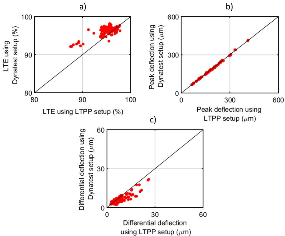
Figure 4-2: Dynatest vs. LTPP Recommended FWD Geophones Layouts a) LTE, b) Peak Deflection, and c) Differential Deflection.
