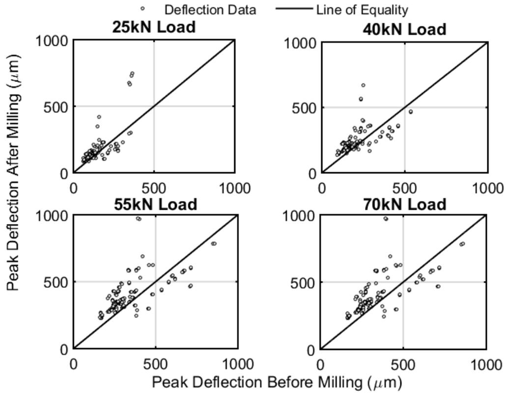
Figure 4-15: Relationship Between Peak Deflections Before and After Milling at Different Loads.
