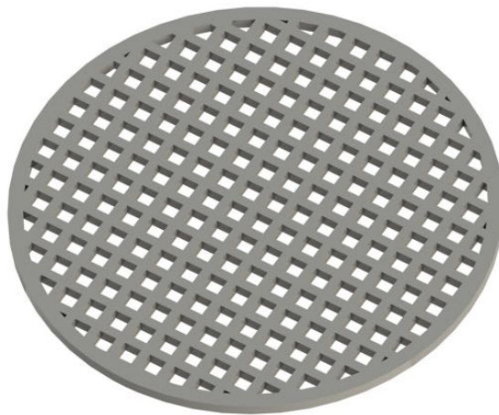
Figure 1: Bed support CAD model used for analysis.
