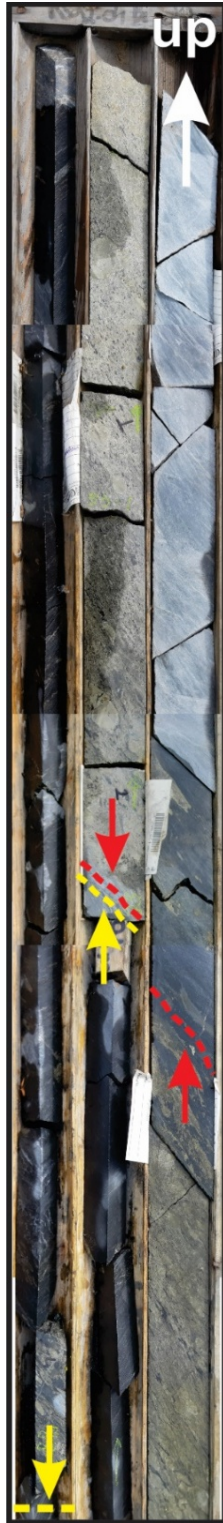
Figure 2.5: Representative photographs of drill core from the Rockstone property; DDH RS22-04. NQ drill core: width = 5 cm. Graphitic intervals are shown by yellow markings and massive sulfide zone is shown by red markings.
