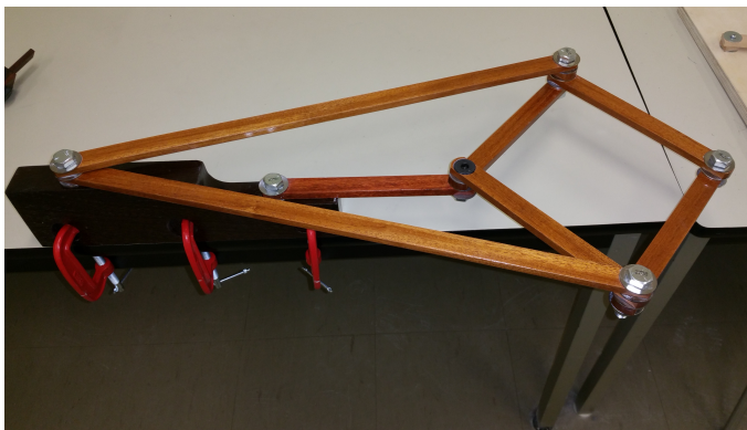
Figure 1.38: Peaucellier's linkage, mahogany and wenge, DSG 2016
